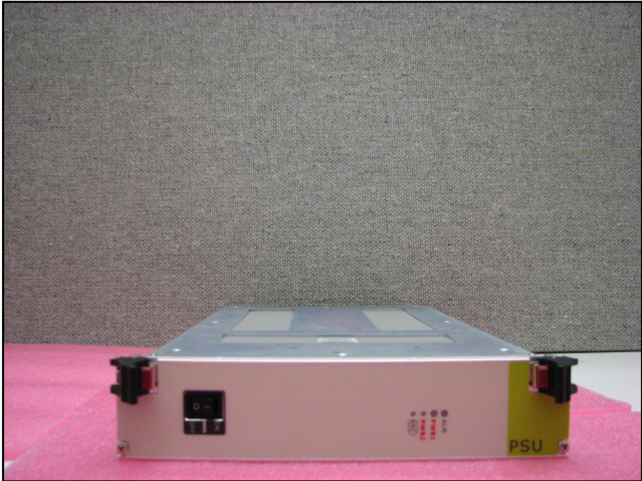
Photograph 13: Power Supply Front
