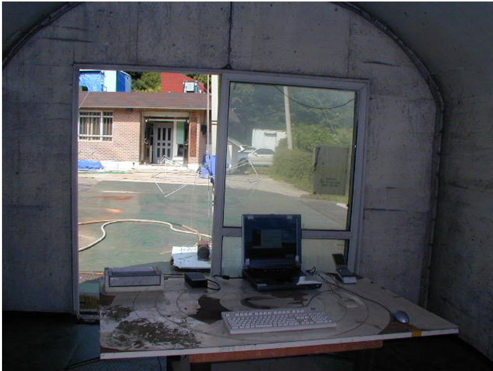
RADIATED EMISSION SETUP PHOTOGRAPH - FRONT VIEW ( 30 - 300 MHz )
