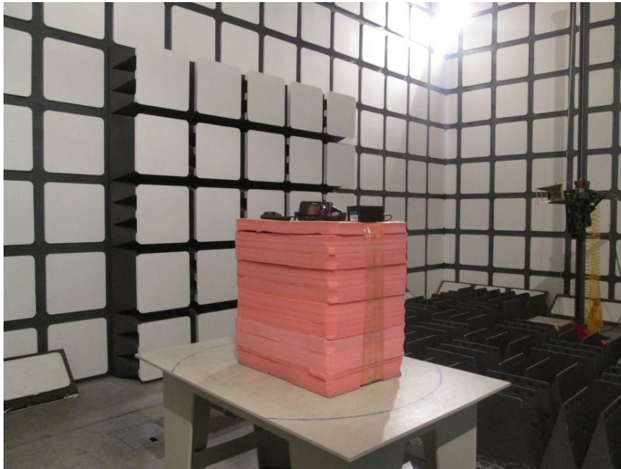
Transmitting Radiated Emissions (Above 1 GHz)
