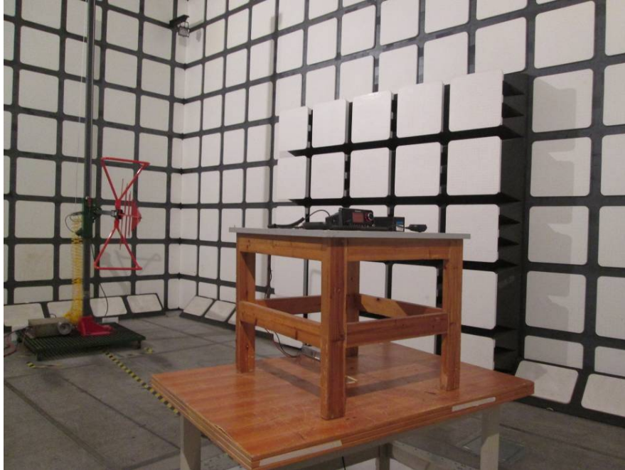
Transmitting Radiated Emissions (Below 1 GHz)
