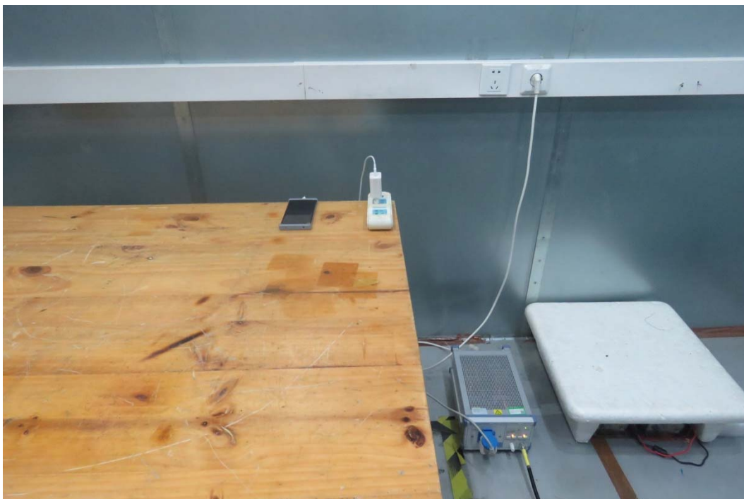
Picture 2 Conducted Emission Test Setup
