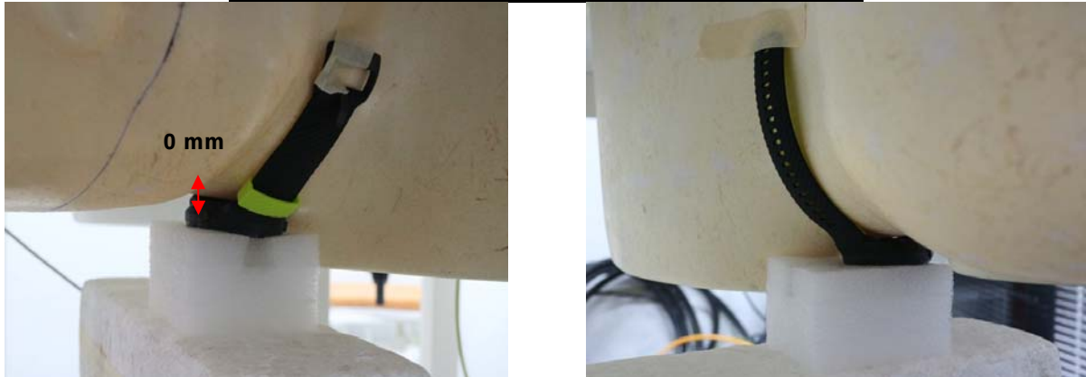
Fig.3 Back side of EUT to flat phantom
