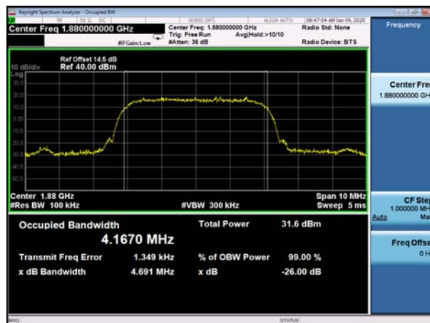
(Plot F2: WCDMA 1900MHz Channel = 9400 Occupied bandwidth)
