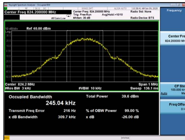
(Plot A1: GSM 850MHz Channel = 128 Occupied bandwidth)
