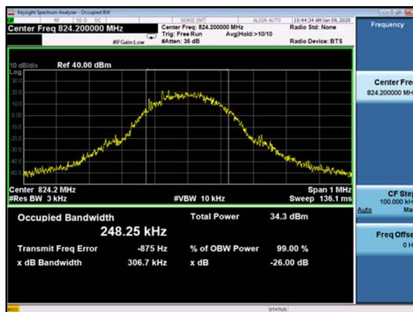
(Plot C1: EDGE 850MHz Channel = 128 Occupied bandwidth)
