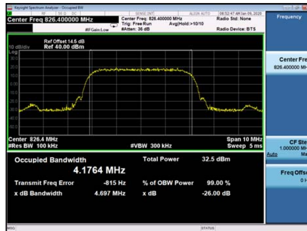
(Plot E1: WCDMA 850MHz Channel = 4132 Occupied bandwidth)
