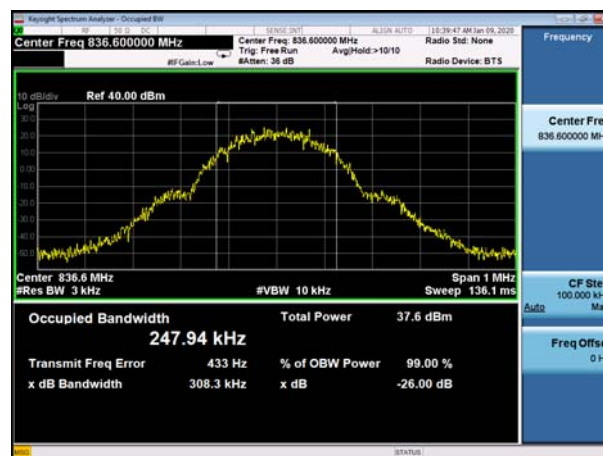
(Plot A2: GSM 850MHz Channel = 190 Occupied bandwidth)
