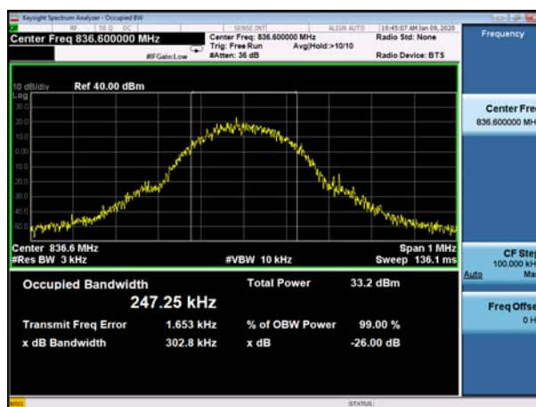
(Plot C2: EDGE 850MHz Channel = 190 Occupied bandwidth)
