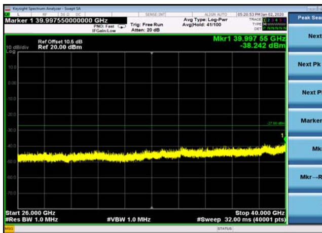
U-NII-1 ,Plot 1,Band Edge-802.11a(20M Hz),5180MHz,Ant1
