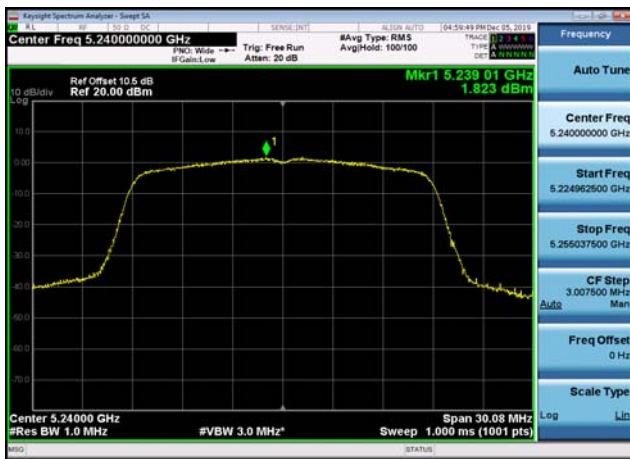
U-NII-1 Power spectral density-802.11 n(40MHz),5230MHz,Ant1
