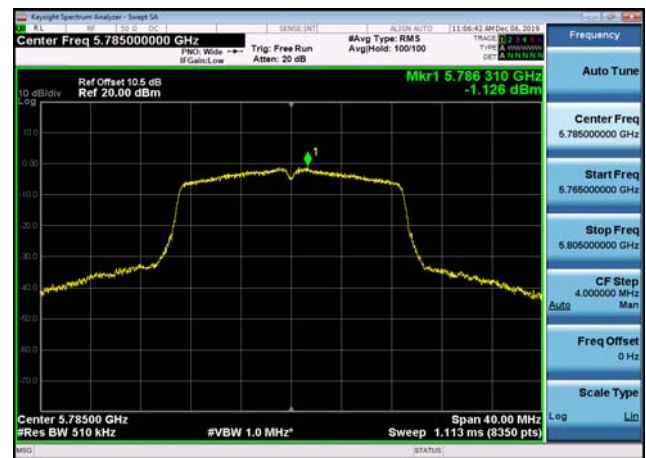
U-NII-3 Power spectral density-802.11 ac(20MHz),5785MHz,Ant1
