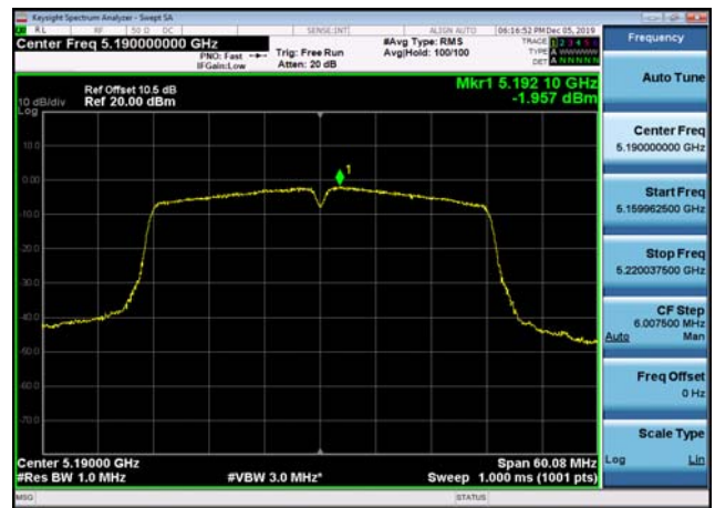
U-NII-1 Power spectral density-802.11 a(20MHz),5180MHz,Ant1
