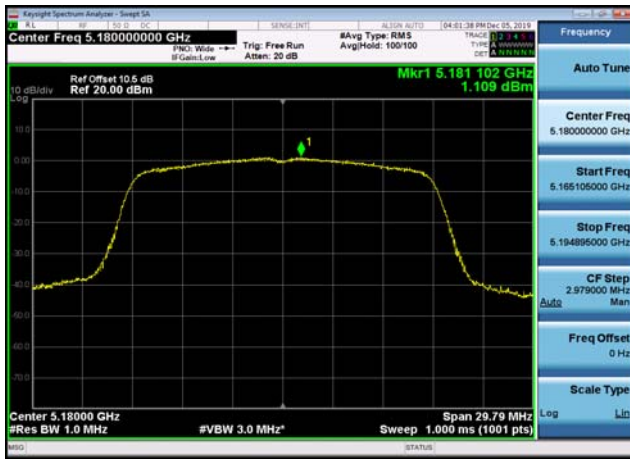
U-NII-1 Power spectral density-802.11 n(20MHz),5240MHz,Ant1
