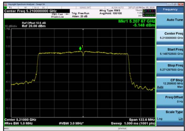
U-NII-1 Power spectral density-802.11 ac(80MHz),5210MHz,Ant1
