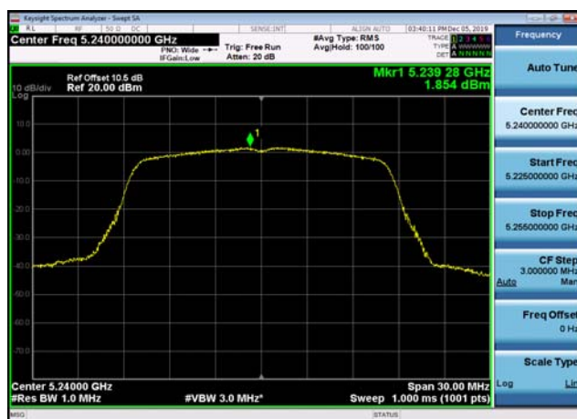
U-NII-1 Power spectral density-802.11 ac(20MHz),5220MHz,Ant1
