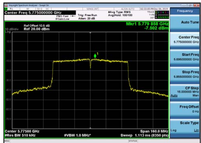
U-NII-3 Power spectral density-802.11 ac(80MHz),5775MHz,Ant1
