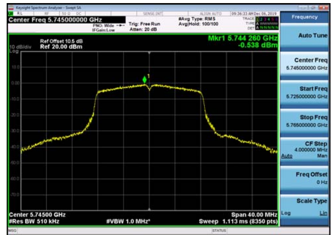
U-NII-3 Power spectral density-802.11 a(20MHz),5825MHz,Ant1
