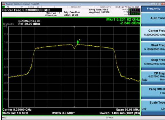
U-NII-1 Power spectral density-802.11 ac(40MHz),5230MHz,Ant1
