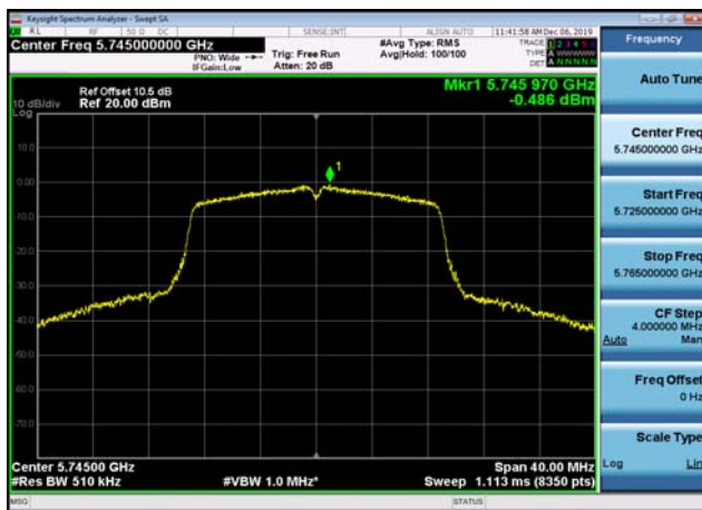
U-NII-3 Power spectral density-802.11 ac(20MHz),5745MHz,Ant1
