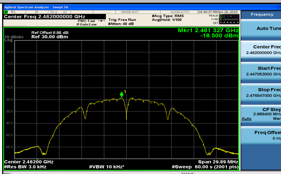
Maximum(average) power spectral density_11B_2462_Ant1
