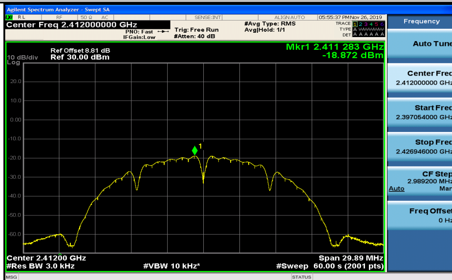
Maximum(average) power spectral density_11B_2437_Ant2
