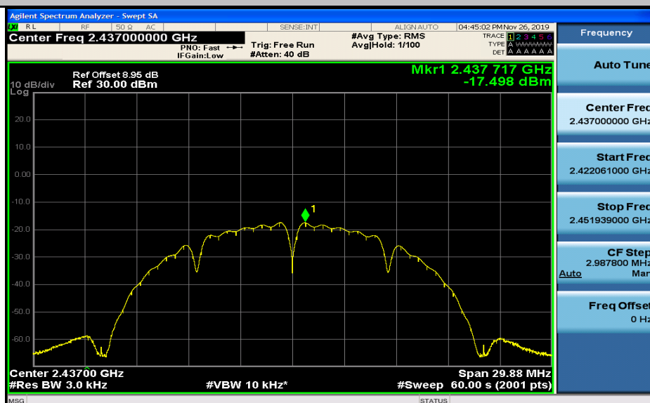
Maximum(average) power spectral density_11B_2462_Ant1
