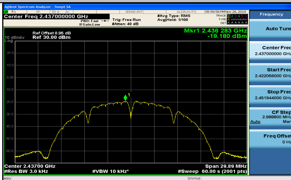
Maximum(average) power spectral density_11B_2462_Ant2
