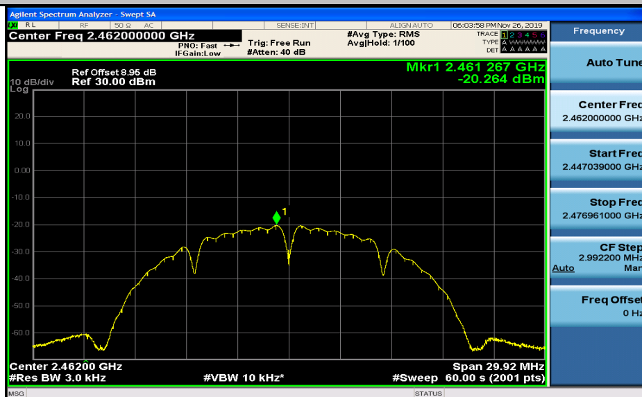
Maximum(average) power spectral density_11B_2462_Ant2
