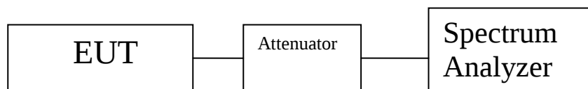
Figure 3. Power Spectral Density Test Setup
