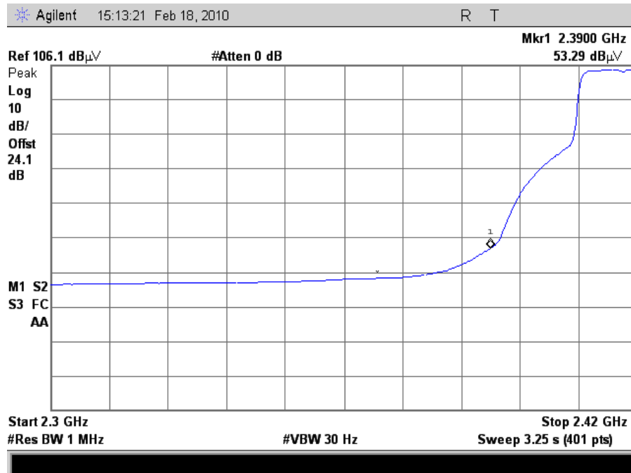
Plot 76. 802.11g Lower Band Edge, Channel 2, Average (6dBi Omni Antenna)
