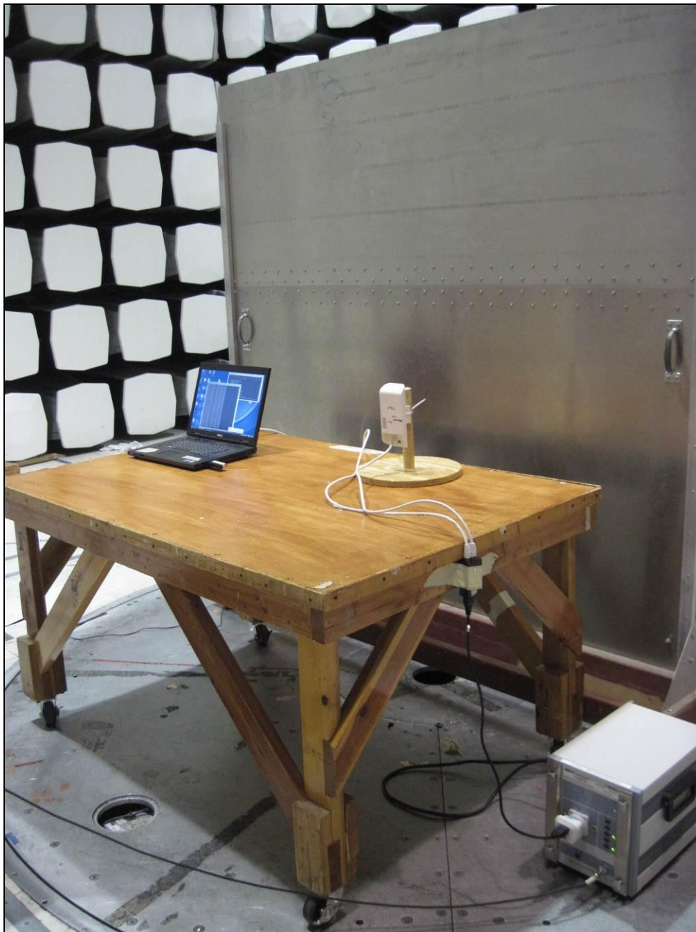
Photograph 2. Conducted Emissions, Test Setup
