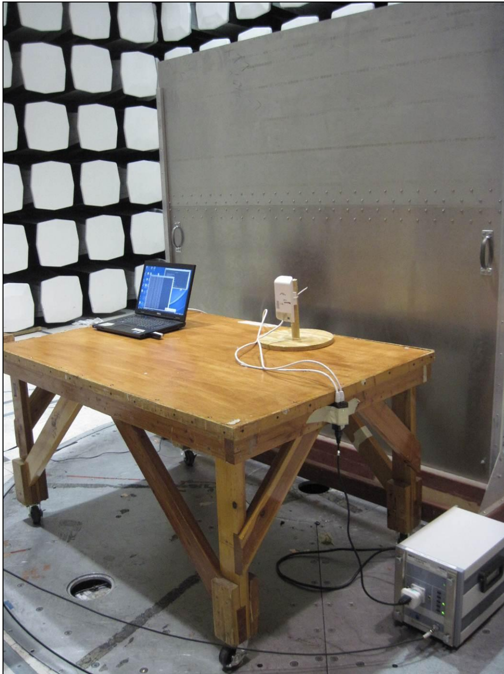
Photograph 4. Conducted Emissions, 15.207(a), Test Setup
