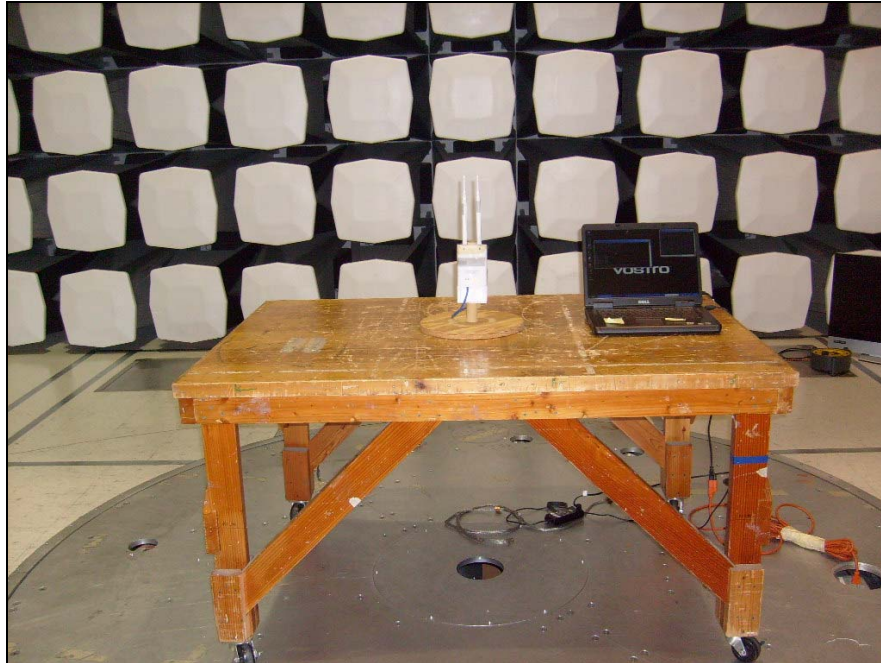
Photograph 3. Radiated Emission, Test Setup
