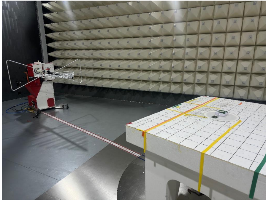
Photograph 1: View Test Set Up Radiated Emissions 30 – 1000 MHz
