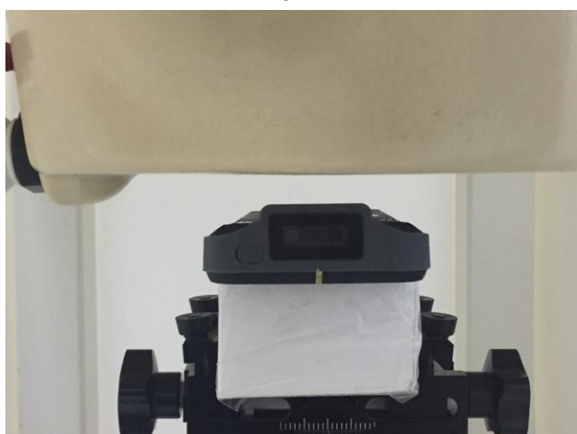
Back, Test Separation 10 mm for WLAN
