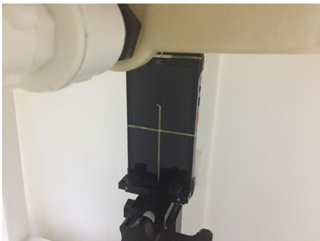
Top Side, Test Separation 0 mm
