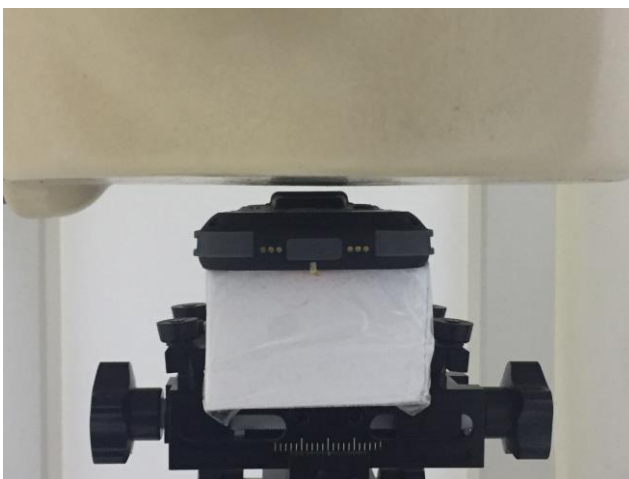
Back, Test Separation 10 mm for WWAN
