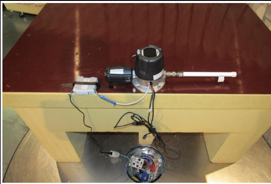
Testsetup below 1GHz EUT view
