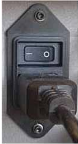
Figure 4-2 Main power switch and cable
