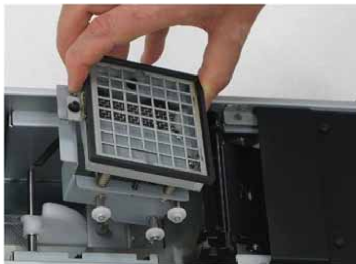
Figure 4-42 Purge unit waste collector
