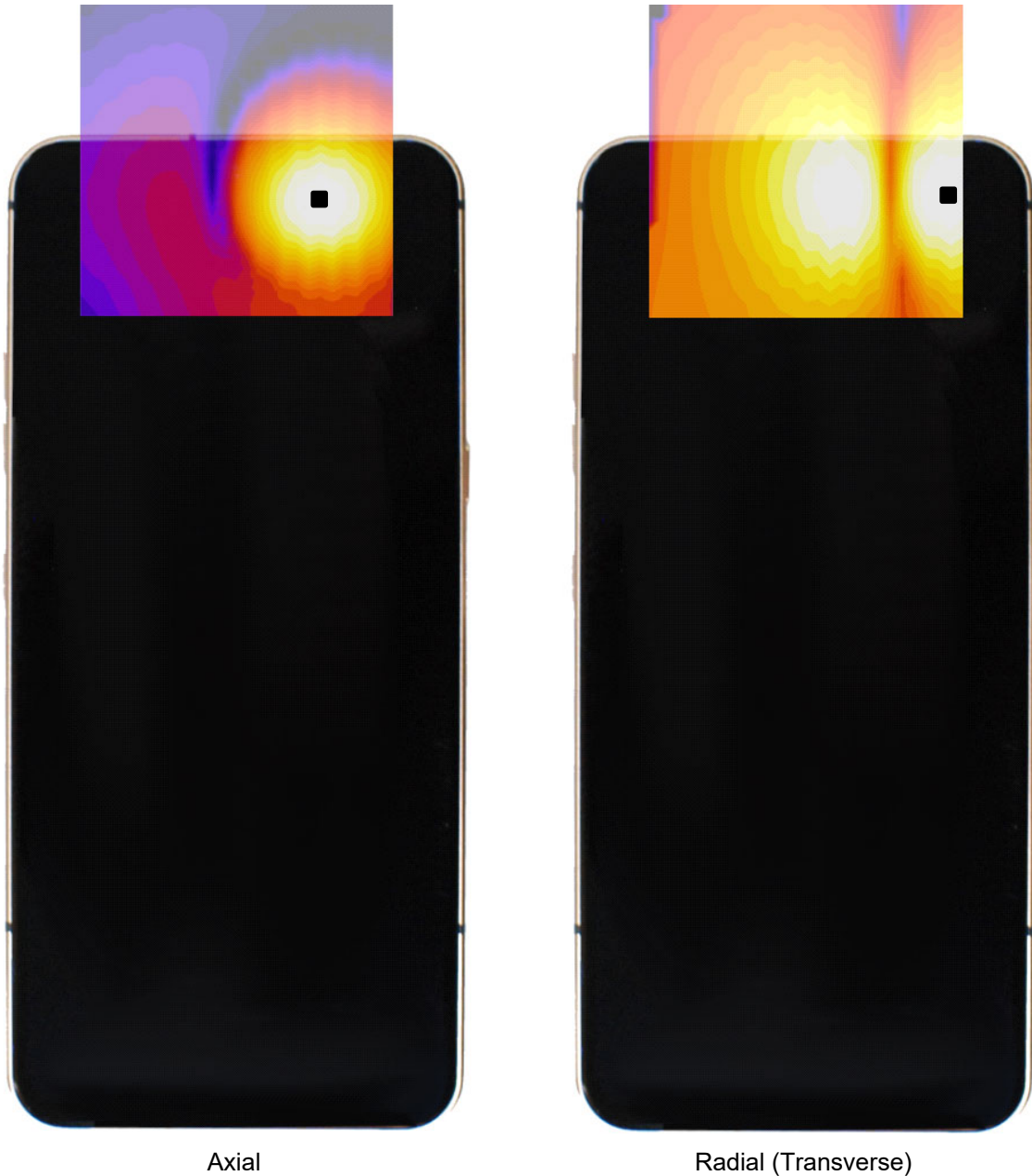
Figure 16-3 T-Coil Scan Overlay Magnetic Field Distributions
