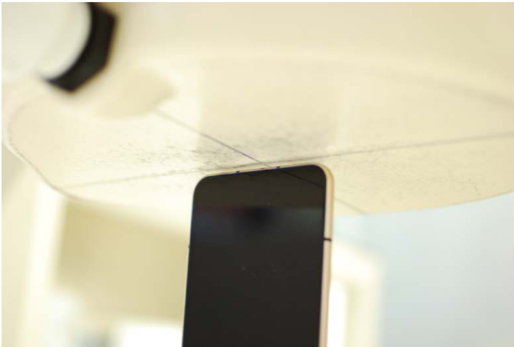
SAR Test Setup Photo 14 – Bottom Edge at 3 mm
