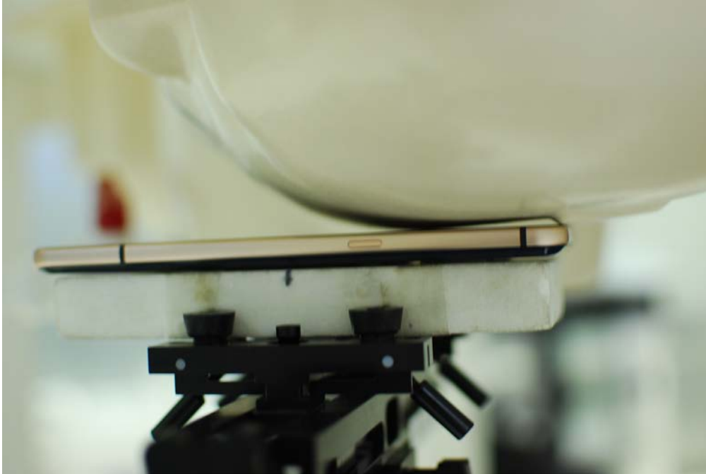
SAR Test Setup Photo 3 – Left Cheek
