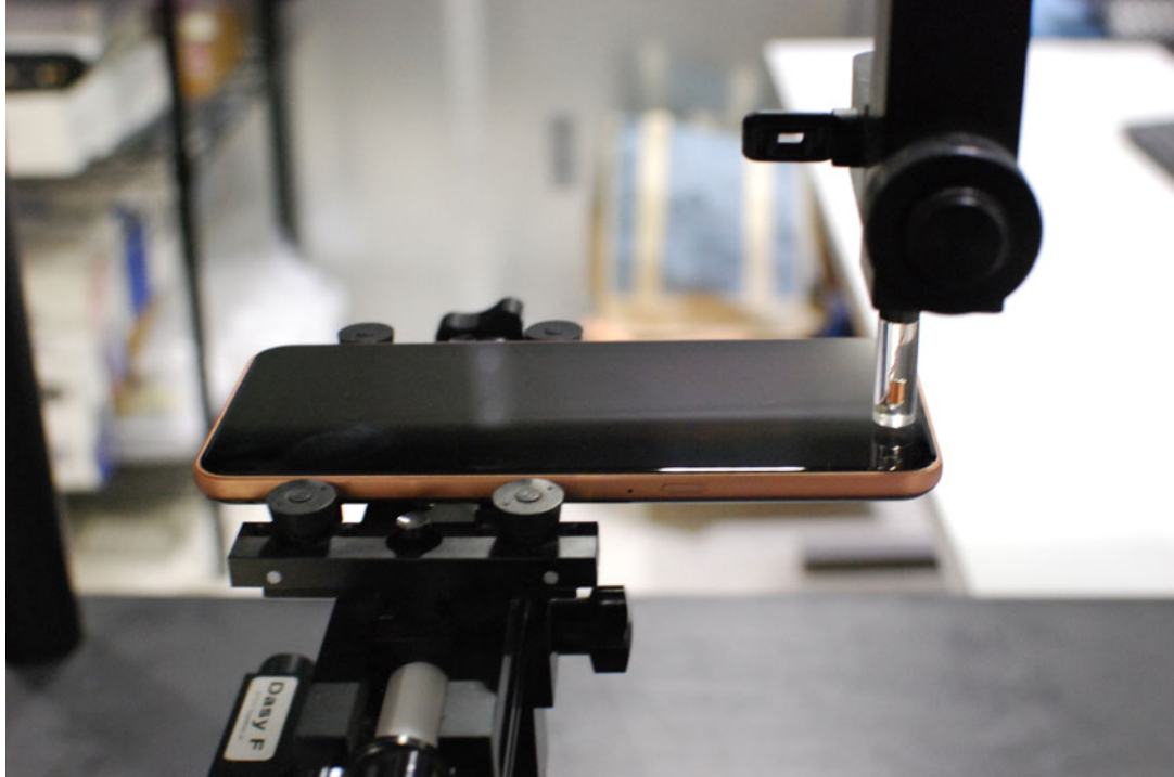
Figure 16-1 Test Setup for Wireless Device
