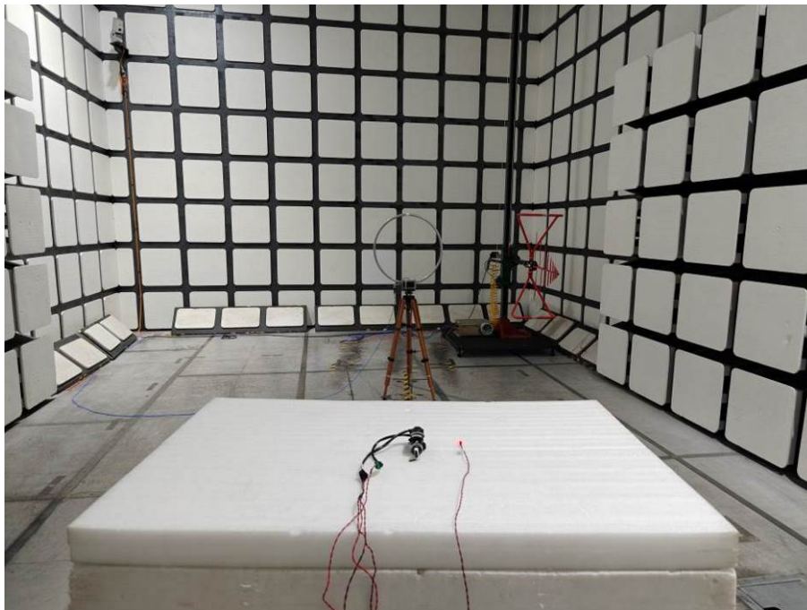
Radiated Emissions View (9 kHz-30 MHz) - Parallel
