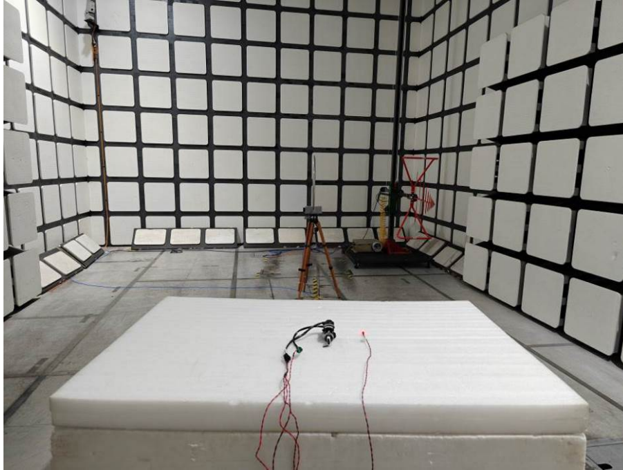
Radiated Emissions View (9 kHz-30 MHz) - Perpendicular
