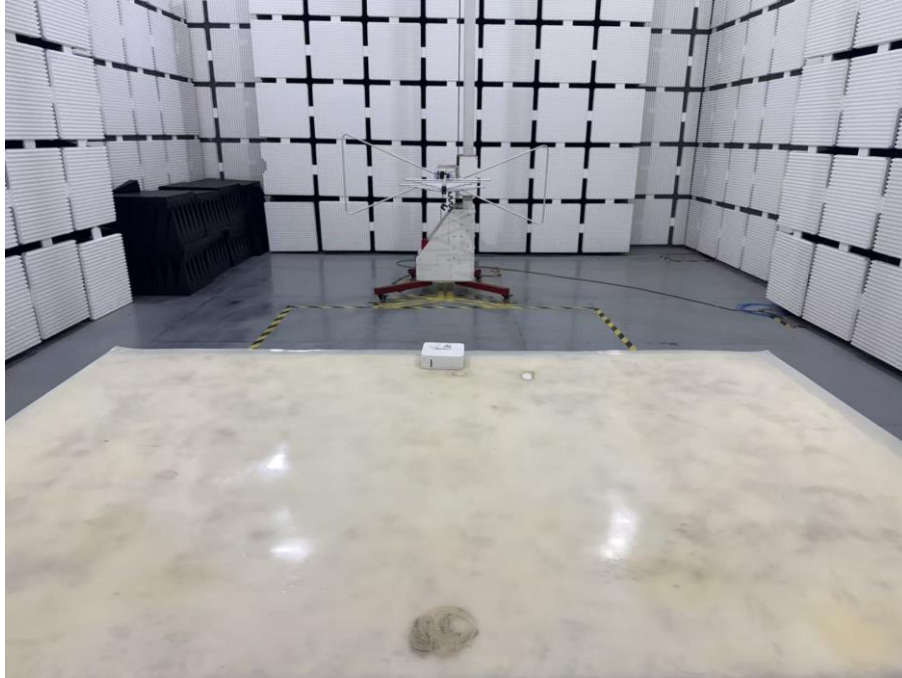
Set-up for Radiated Spurious Emission, Above 1GHz
