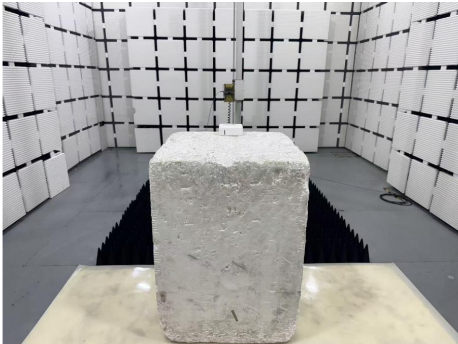
Set-up for Radiated Spurious Emission, Above 1GHz
