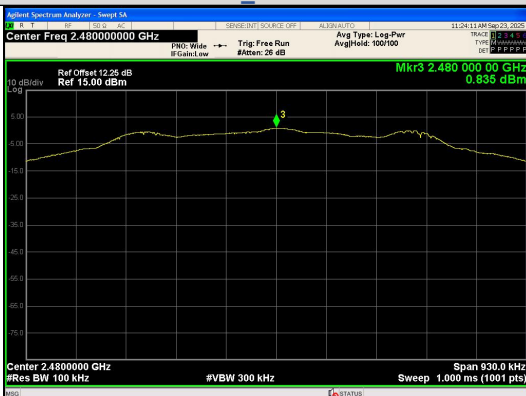
In-Band Reference Level BLE 1M_Channel 39
