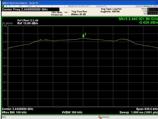
In-Band Reference Level BLE 1M_Channel 19
