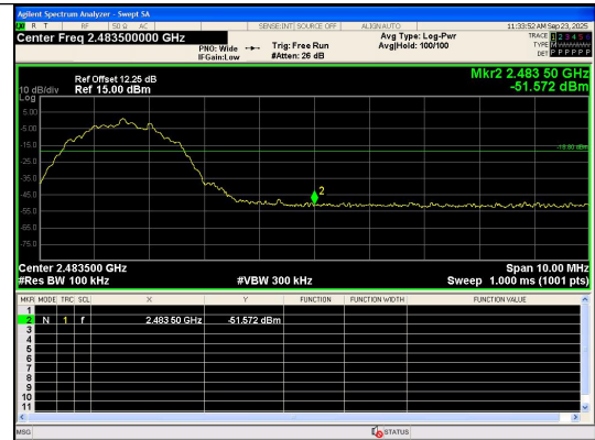
Out Of Band Emission BLE 2M_Channel 39
