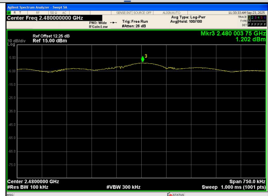
In-Band Reference Level BLE 2M_Channel 39
