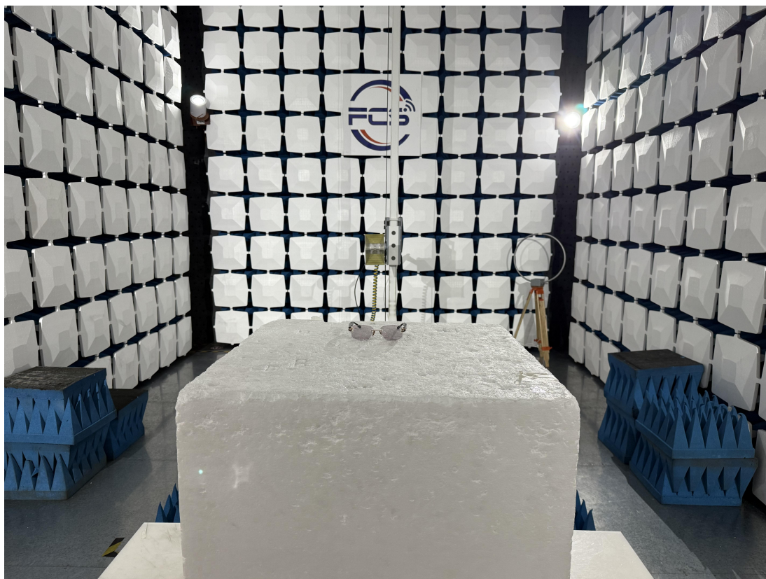
Above 1GHz for radiated emission test setup
