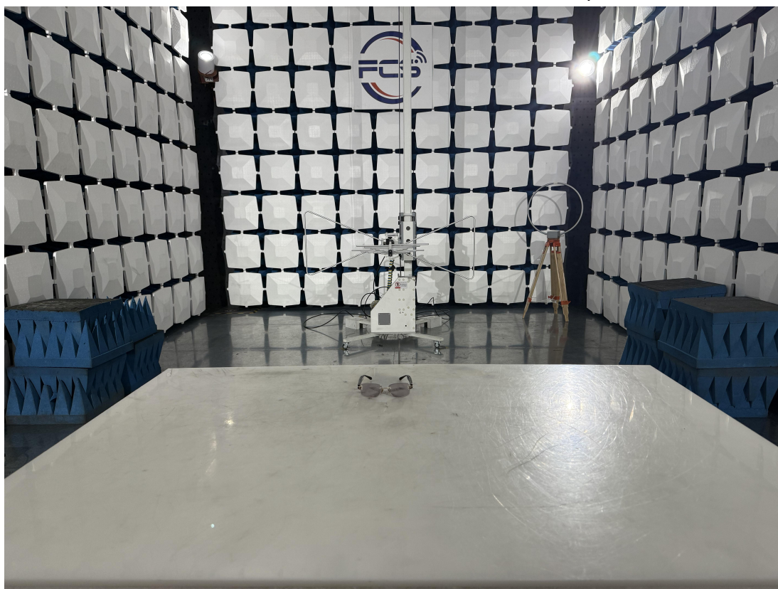
Above 1GHz for radiated emission test setup
