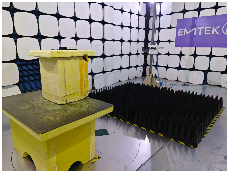
Spurious Emission Test Setup (Above 1GHz)
