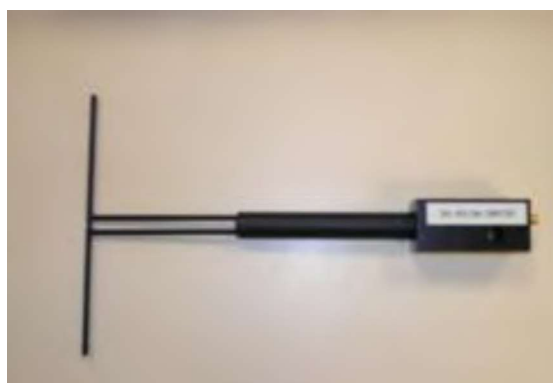
Figure 1 – MVG COMOSAR Validation Dipole
