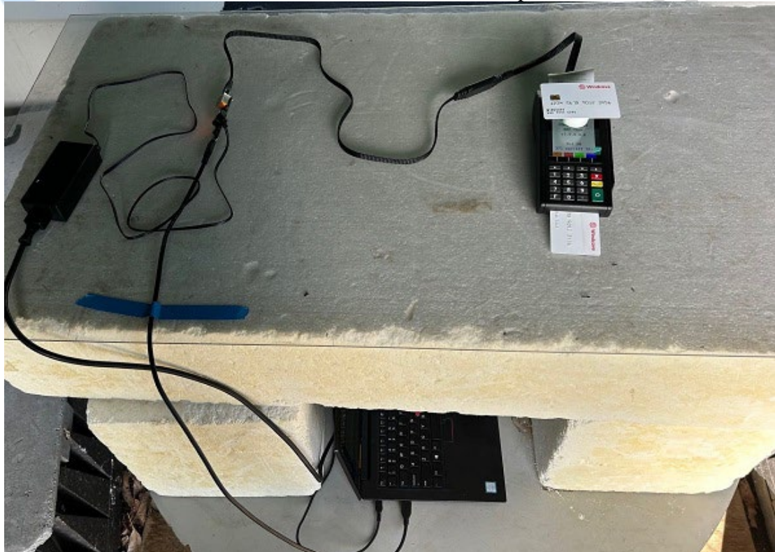
Radiated Emissions Test Setup
