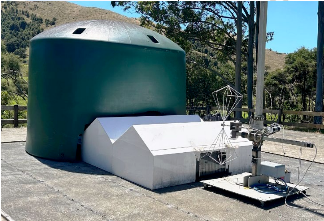
Radiated Emissions Test Setup - Biconical Antenna
