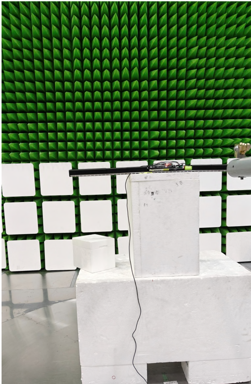
Figure 5 – Radiated Emissions Setup 18GHz – 40GHz
