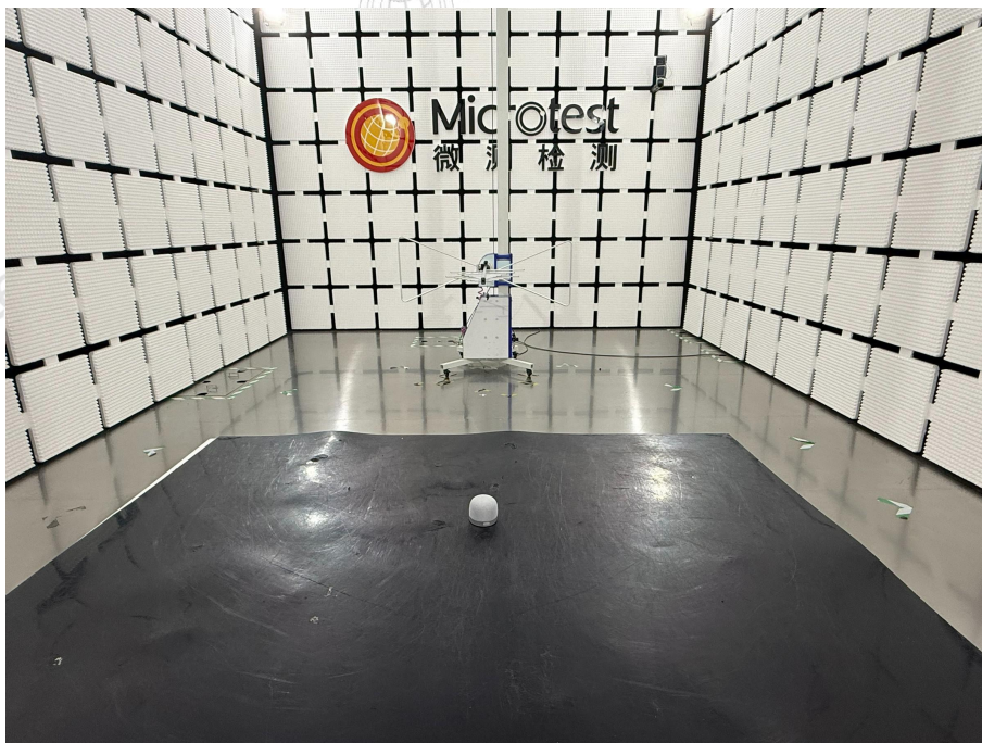
Radiated emissions (below 1GHz) -BT&BLE
