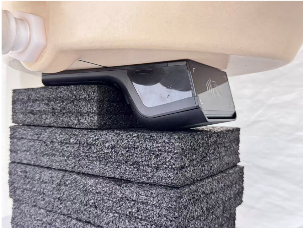
Picture 9: Front Side, the distance from EUT to the bottom of the Phantom is 0mm
