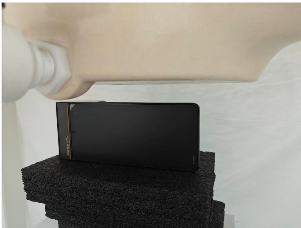
Picture 14: Right Edge, the distance from EUT to the bottom of the Phantom is 24mm
