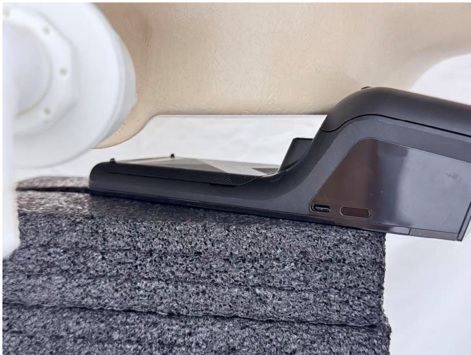
Picture 13: Back Side, the distance from EUT to the bottom of the Phantom is 14mm
