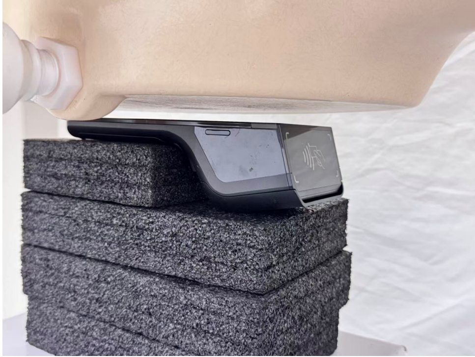
Picture 3: Front Side, the distance from EUT to the bottom of the Phantom is 10mm
