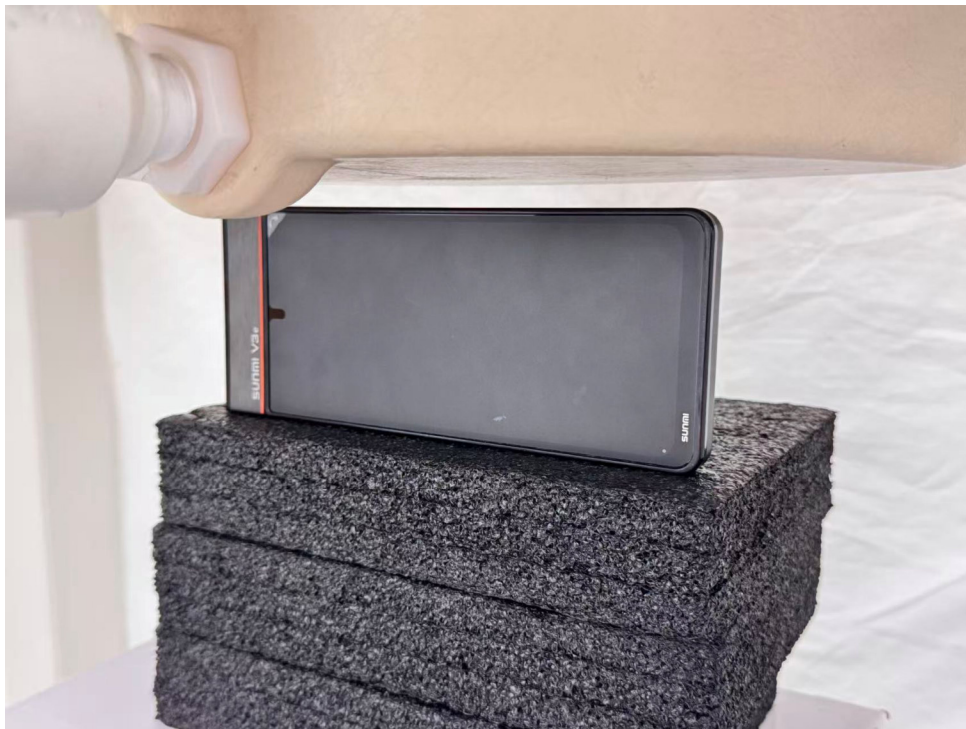
Picture 5: Right Edge, the distance from EUT to the bottom of the Phantom is 10mm
