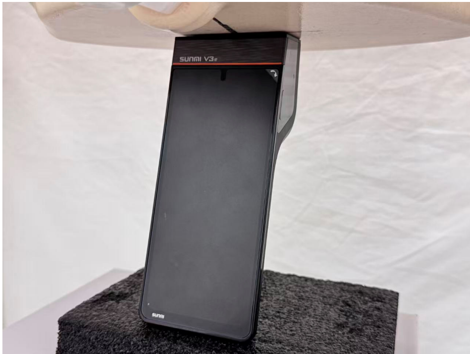
Picture 12: Top Edge, the distance from EUT to the bottom of the Phantom is 0mm
