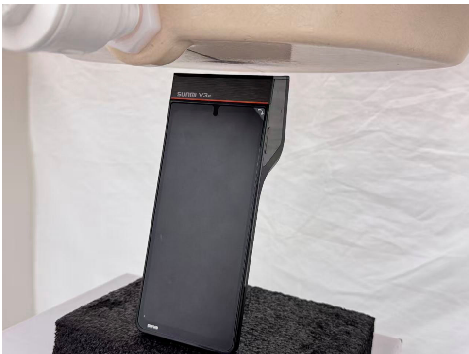
Picture 6: Top Edge, the distance from EUT to the bottom of the Phantom is 10mm
