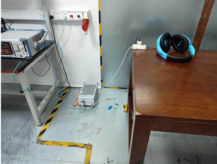
Conducted emissions at AC power line (150kHz-30MHz)
