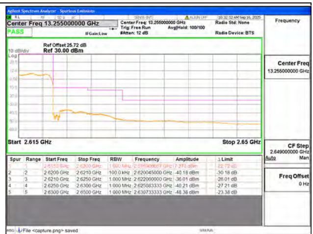
B38 / 10MHz / High CH / QPSK / FULL RB
