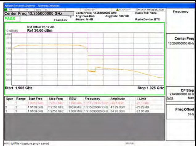
B25 / 10MHz / High CH / QPSK / FULL RB
