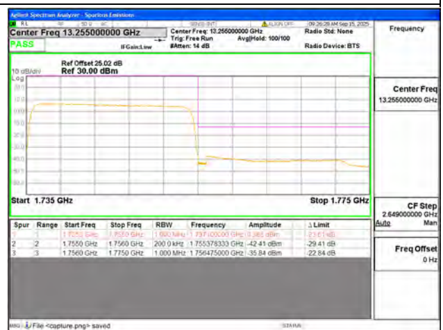
B4 / 20MHz / High CH / QPSK / FULL RB
