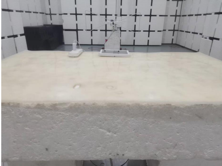
Set-up for Radiated Spurious Emission, Above 1GHz
