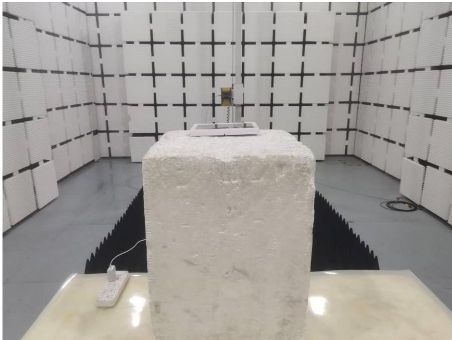
Set-up for Radiated Spurious Emission, Above 1GHz
