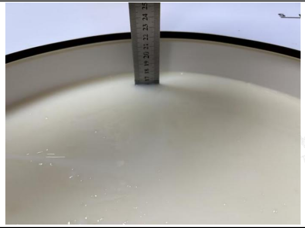
Photo 1: Tissue Simulant Liquid for Head 700- 3000MHz
