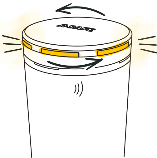
Warning (Spinning Orange Light)
