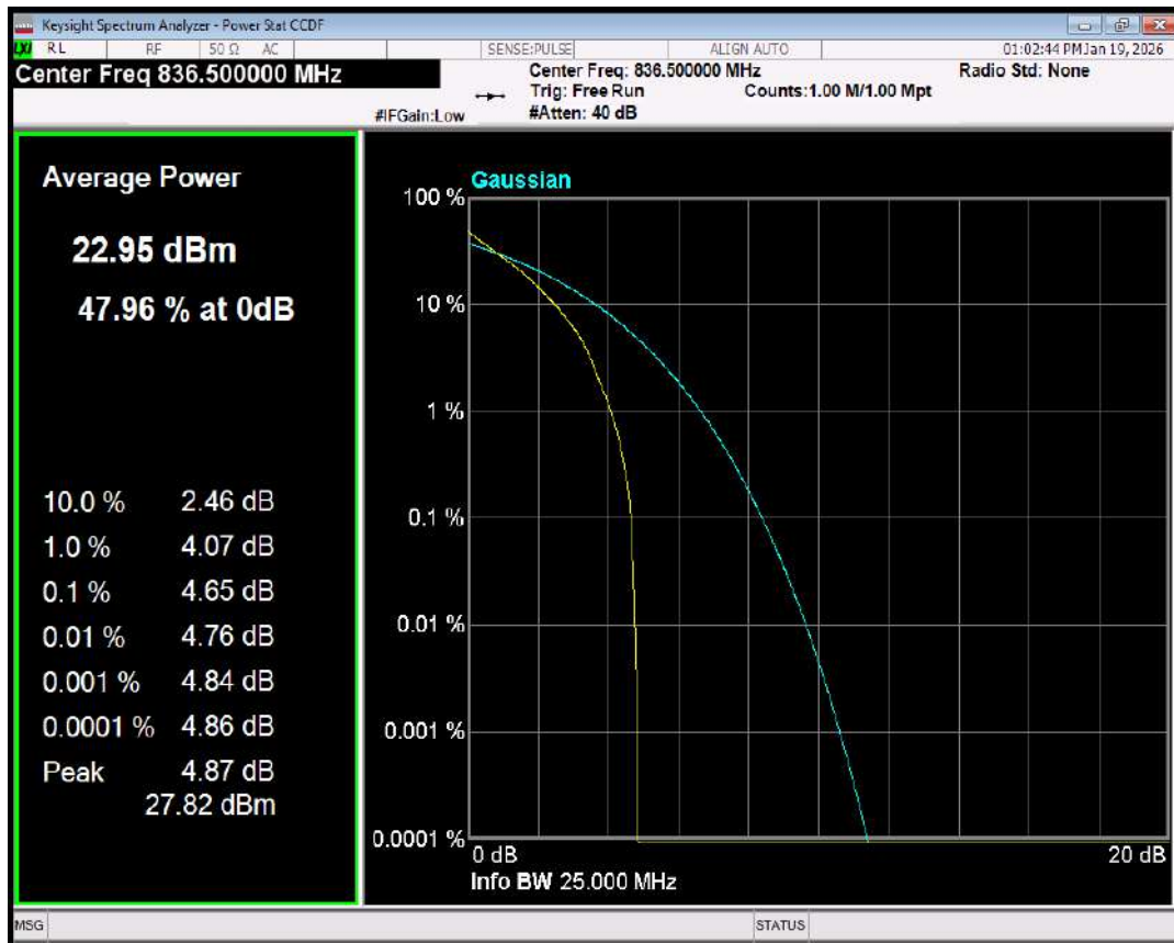
Band5 16QAM BW=10MHz Channel=20525 RB Size=1 Position=#0
