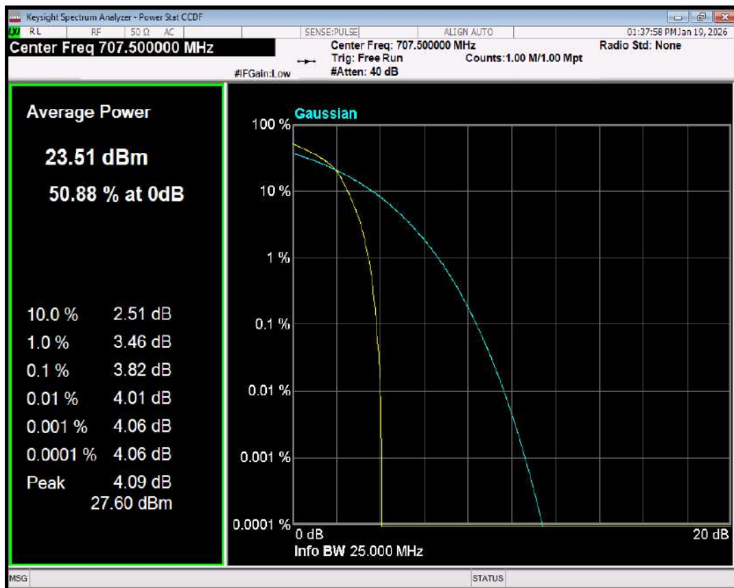
Band12 QPSK BW=3MHz Channel=23095 RB Size=1 Position=#0
