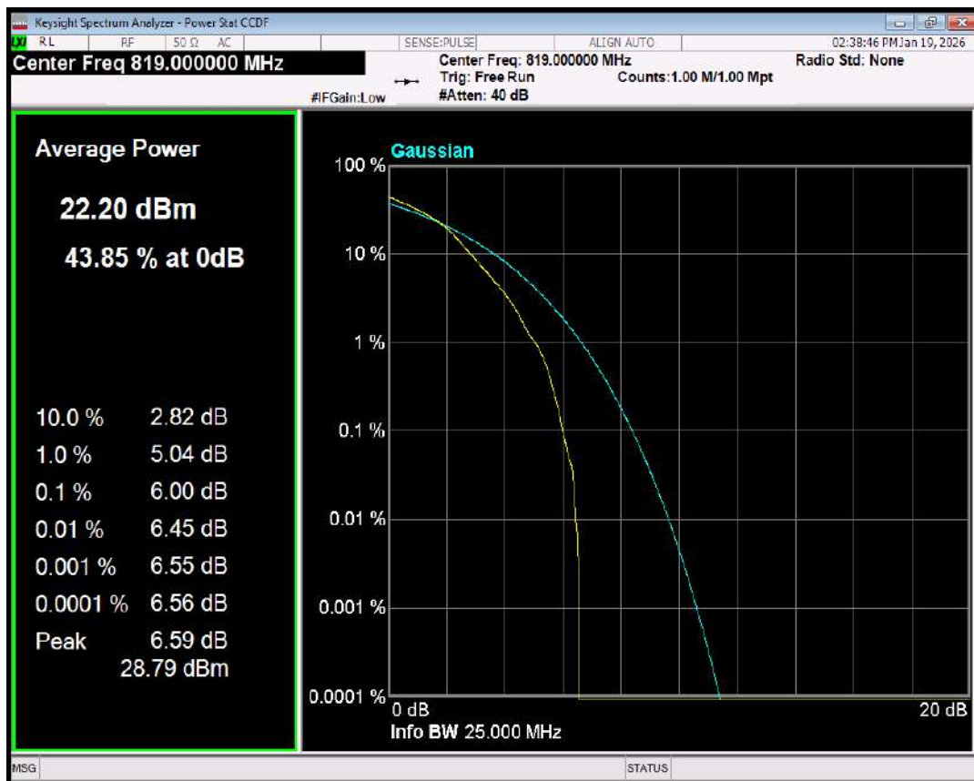
Band26(814-824) QPSK BW=3MHz Channel=26740 RB Size=1 Position=#0
