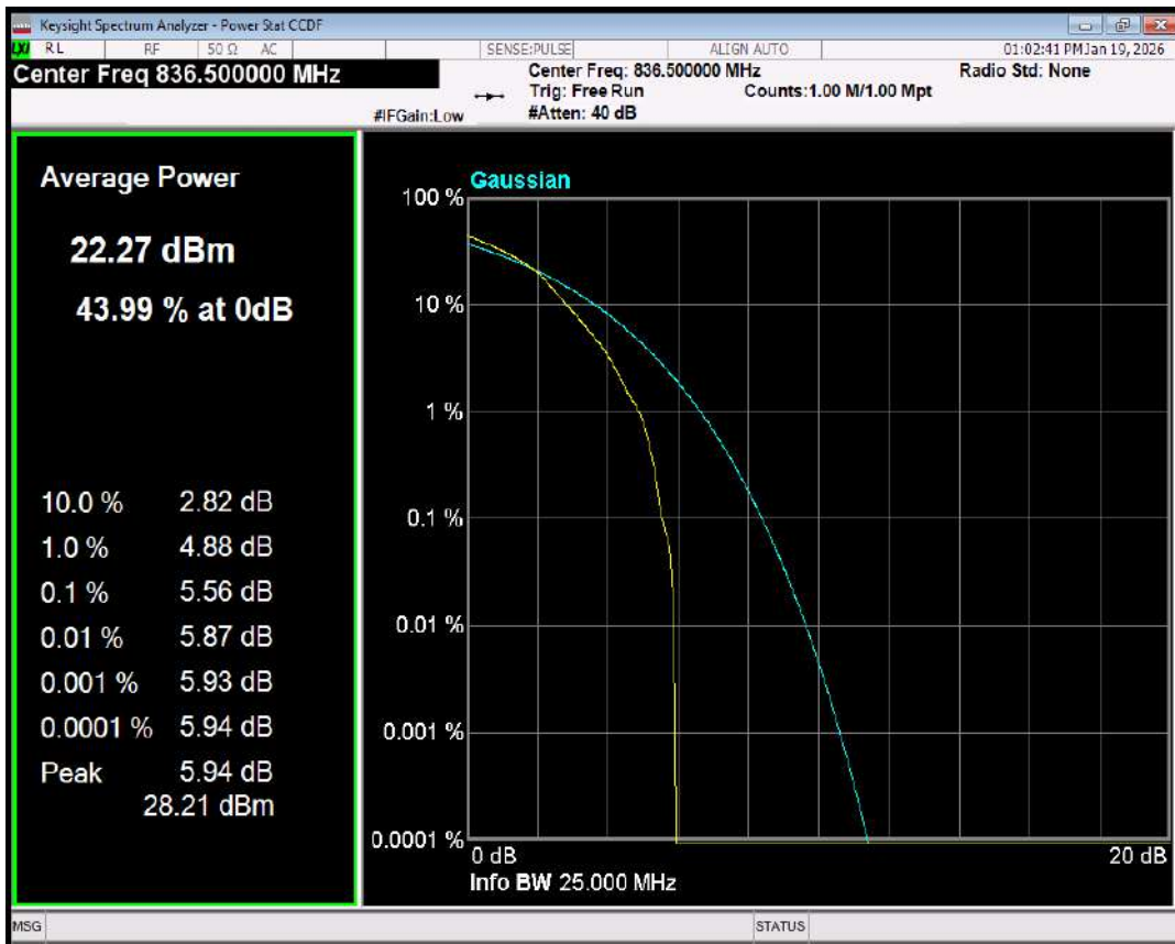
Band5 QPSK BW=10MHz Channel=20525 RB Size=1 Position=#0
