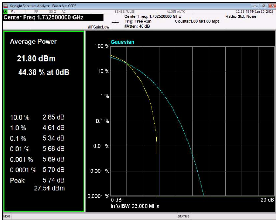
Band4 QPSK BW=10MHz Channel=20175 RB Size=1 Position=#0
