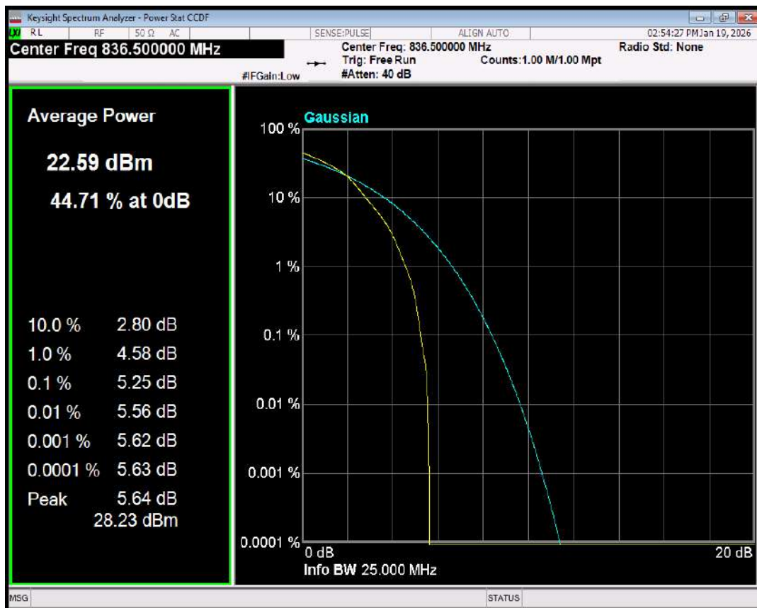
Band26(824-849) QPSK BW=15MHz Channel=26915 RB Size=1 Position=#0
