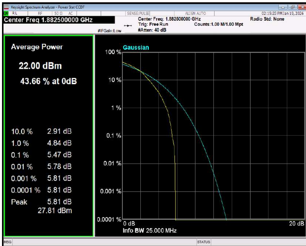
Band25 QPSK BW=10MHz Channel=26365 RB Size=1 Position=#0
