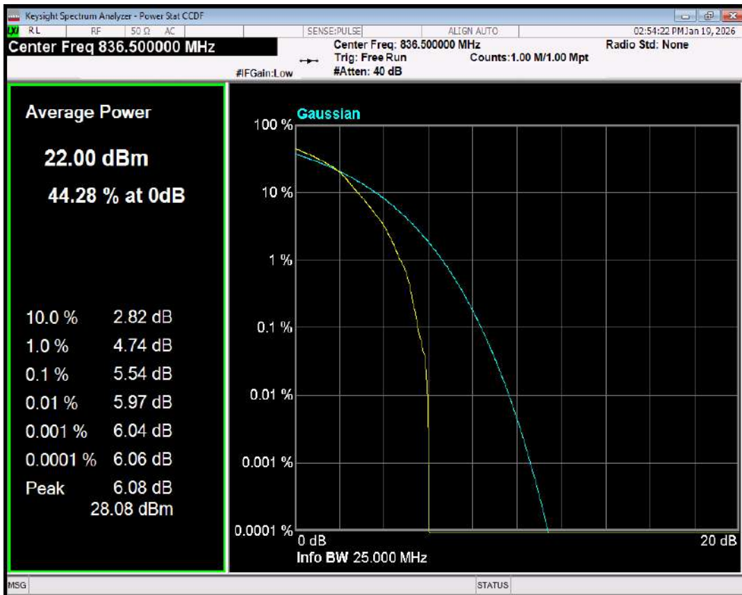
Band26(824-849) QPSK BW=10MHz Channel=26915 RB Size=1 Position=#0
