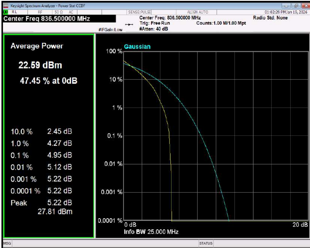
Band5 16QAM BW=1.4MHz Channel=20525 RB Size=1 Position=#0
