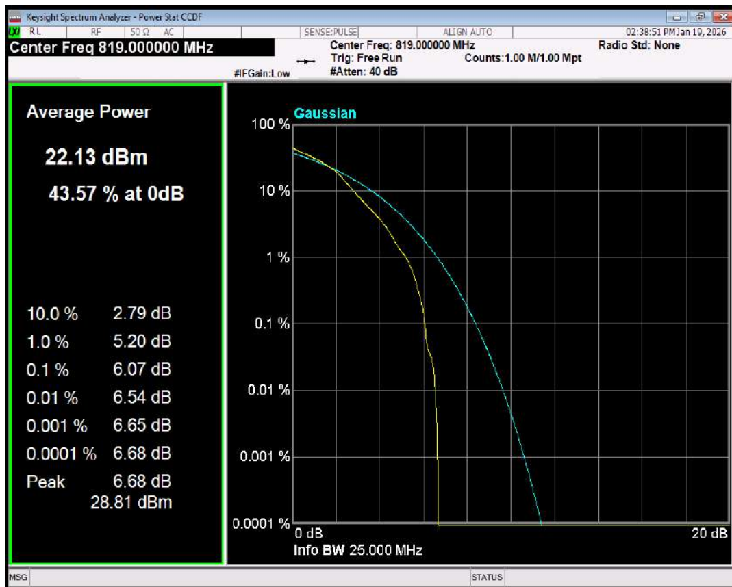
Band26(814-824) QPSK BW=5MHz Channel=26740 RB Size=1 Position=#0
