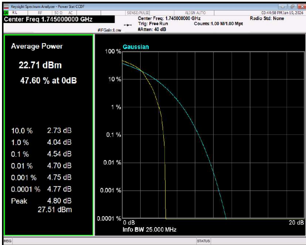
Band66 QPSK BW=20MHz Channel=132322 RB Size=1 Position=#0
