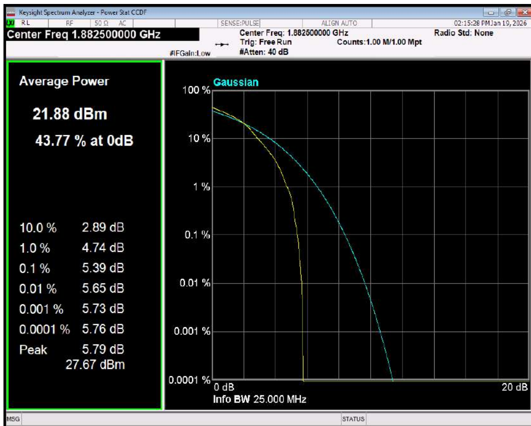
Band25 QPSK BW=15MHz Channel=26365 RB Size=1 Position=#0
