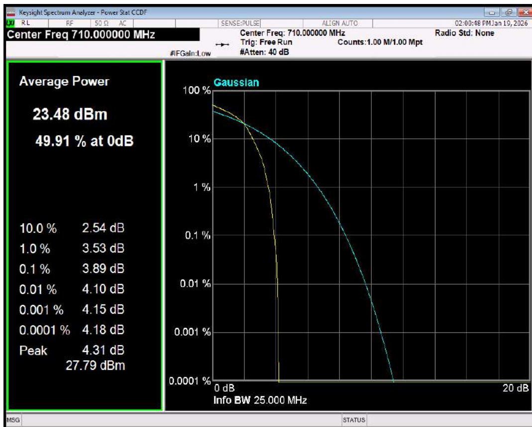
Band17 QPSK BW=10MHz Channel=23790 RB Size=1 Position=#0
