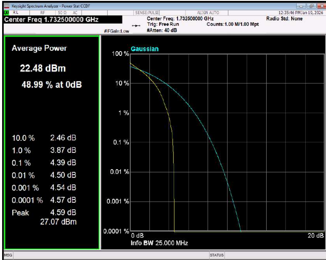
Band4 16QAM BW=5MHz Channel=20175 RB Size=1 Position=#0
