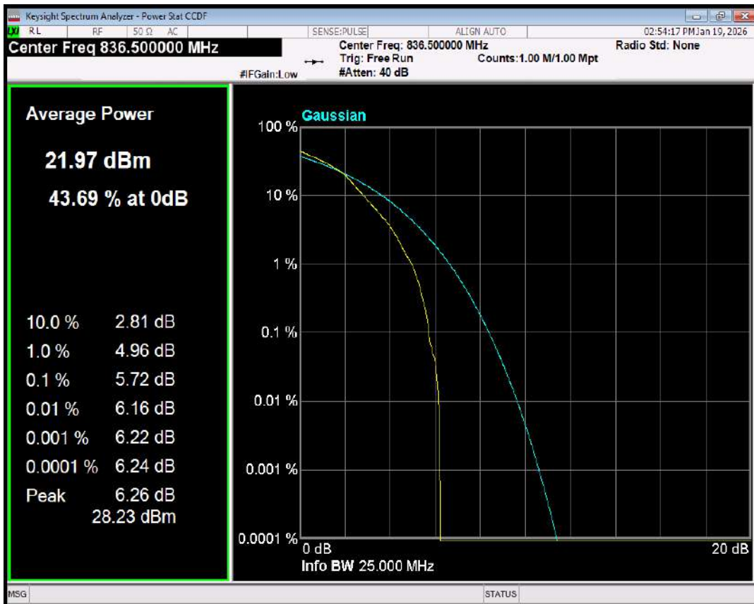
Band26(824-849) QPSK BW=5MHz Channel=26915 RB Size=1 Position=#0
