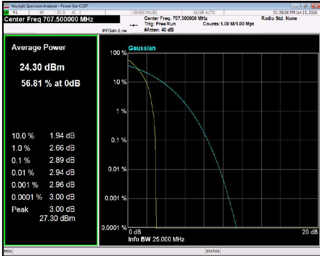
Band12 16QAM BW=5MHz Channel=23095 RB Size=1 Position=#0
