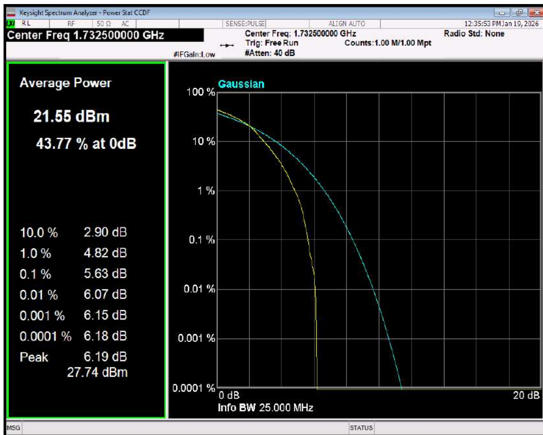
Band4 QPSK BW=15MHz Channel=20175 RB Size=1 Position=#0
