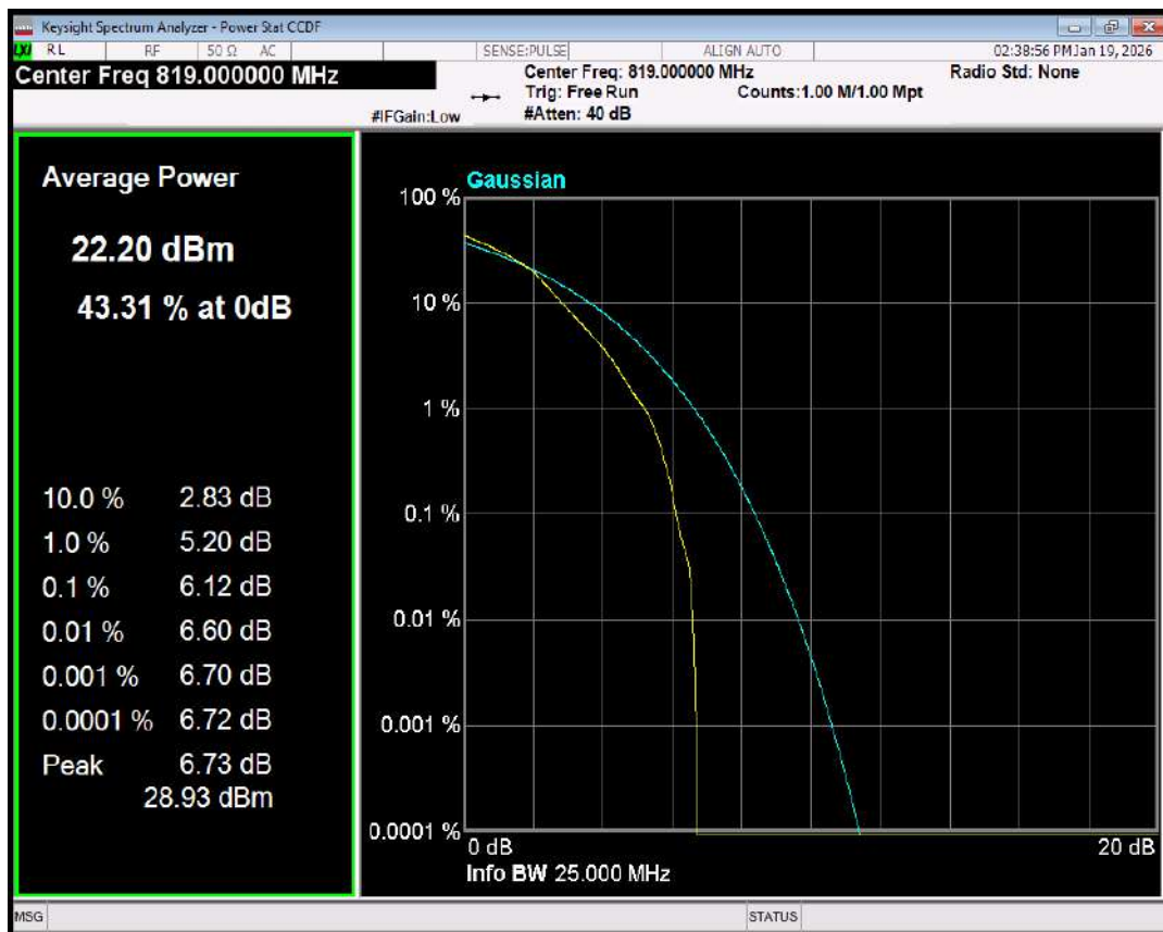
Band26(814-824) QPSK BW=10MHz Channel=26740 RB Size=1 Position=#0
