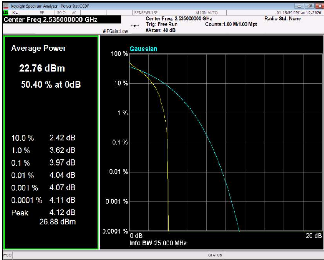
Band7 16QAM BW=5MHz Channel=21100 RB Size=1 Position=#0
