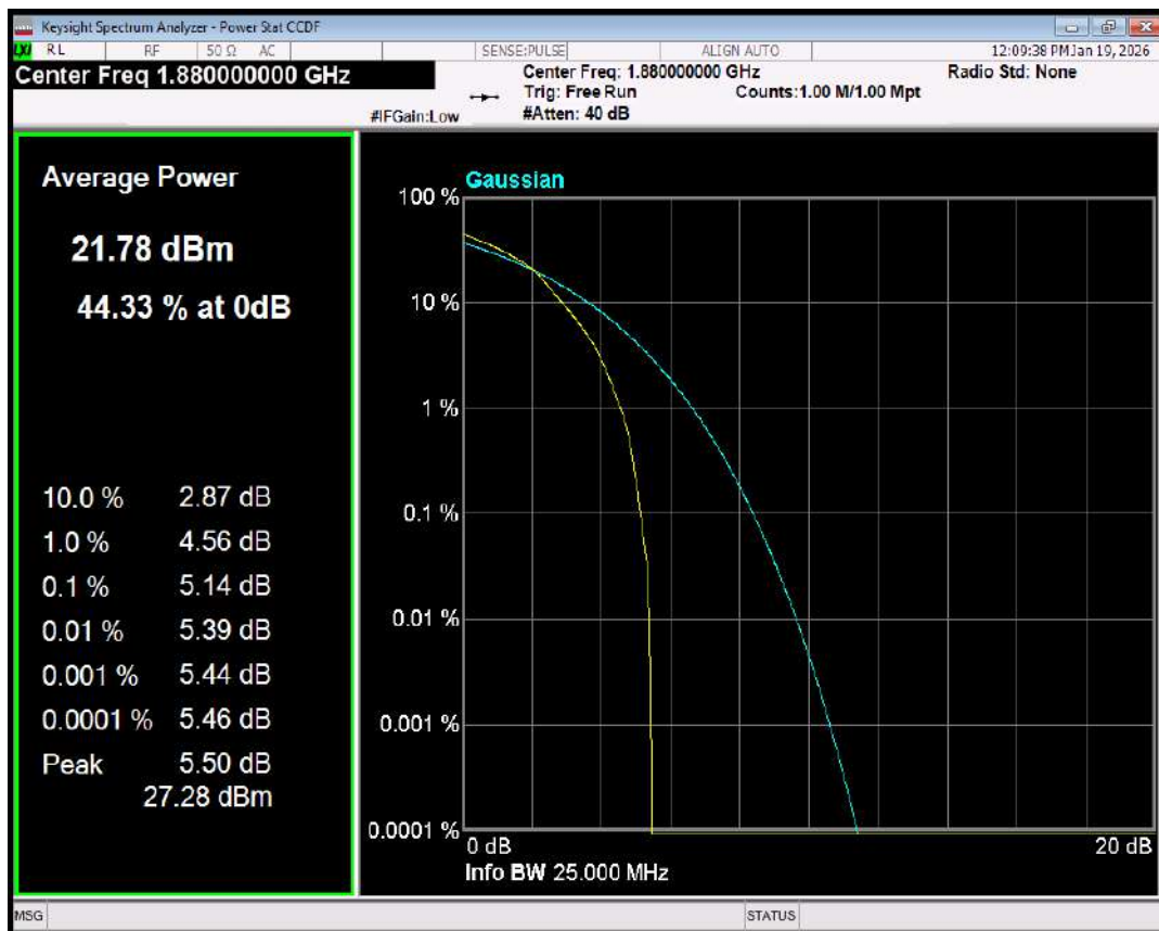
Band2 16QAM BW=20MHz Channel=18900 RB Size=1 Position=#0
