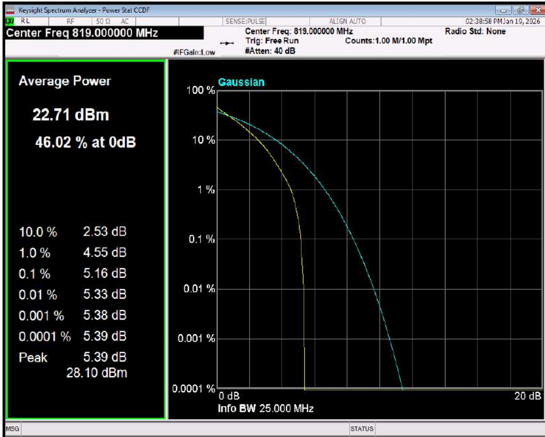
Band26(814-824) 16QAM BW=10MHz Channel=26740 RB Size=1 Position=#0
