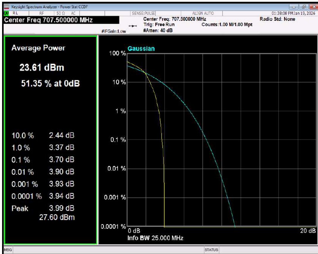
Band12 QPSK BW=10MHz Channel=23095 RB Size=1 Position=#0
