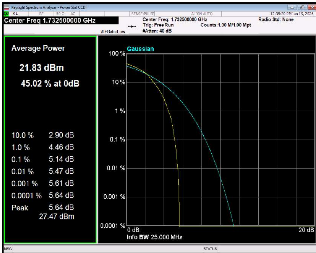
Band4 QPSK BW=3MHz Channel=20175 RB Size=1 Position=#0
