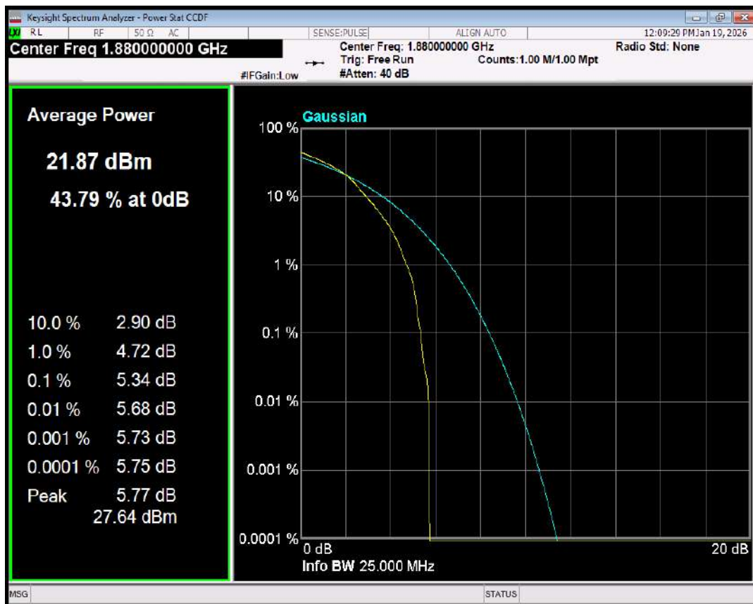
Band2 QPSK BW=10MHz Channel=18900 RB Size=1 Position=#0
