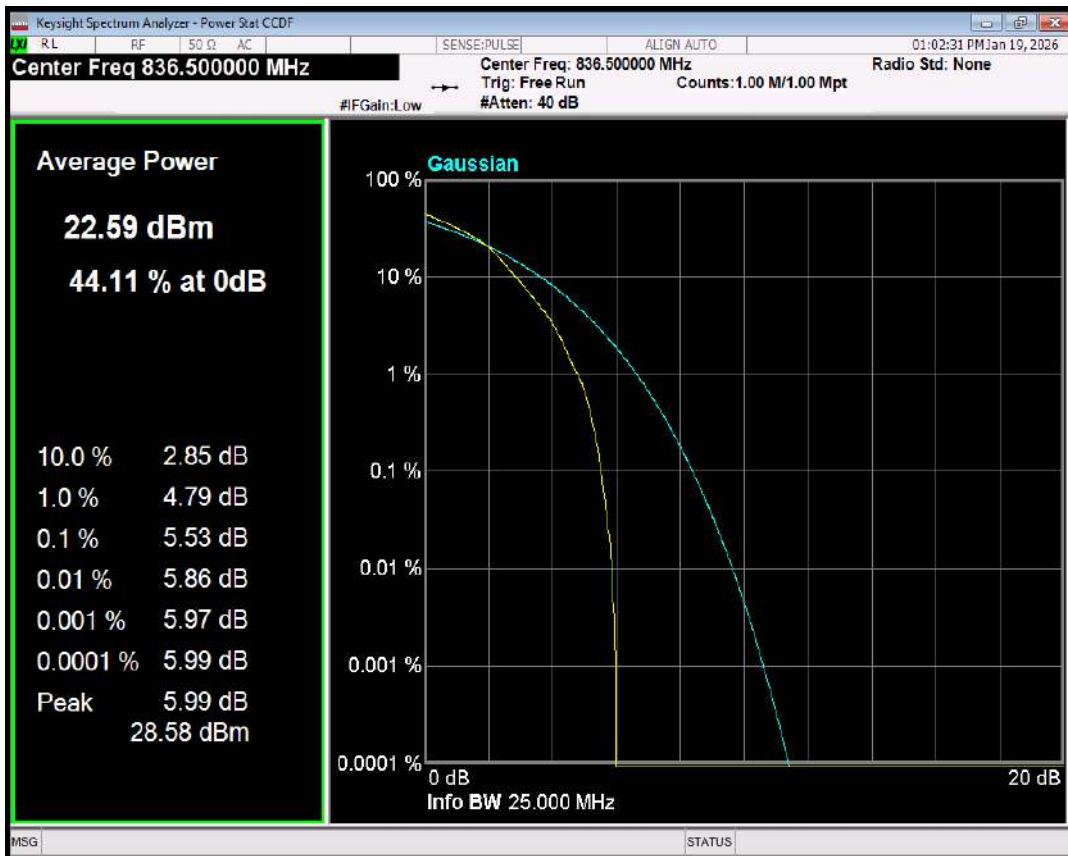
Band5 QPSK BW=3MHz Channel=20525 RB Size=1 Position=#0
