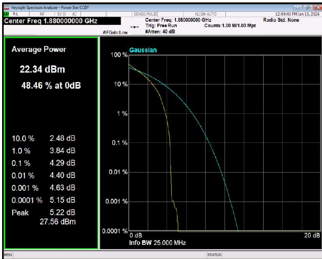
Band25 QPSK BW=1.4MHz Channel=26365 RB Size=1 Position=#0
