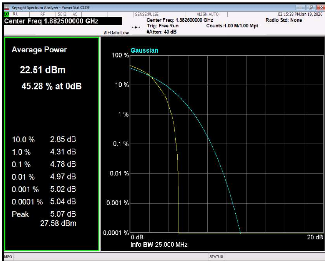
Band25 16QAM BW=20MHz Channel=26365 RB Size=1 Position=#0
