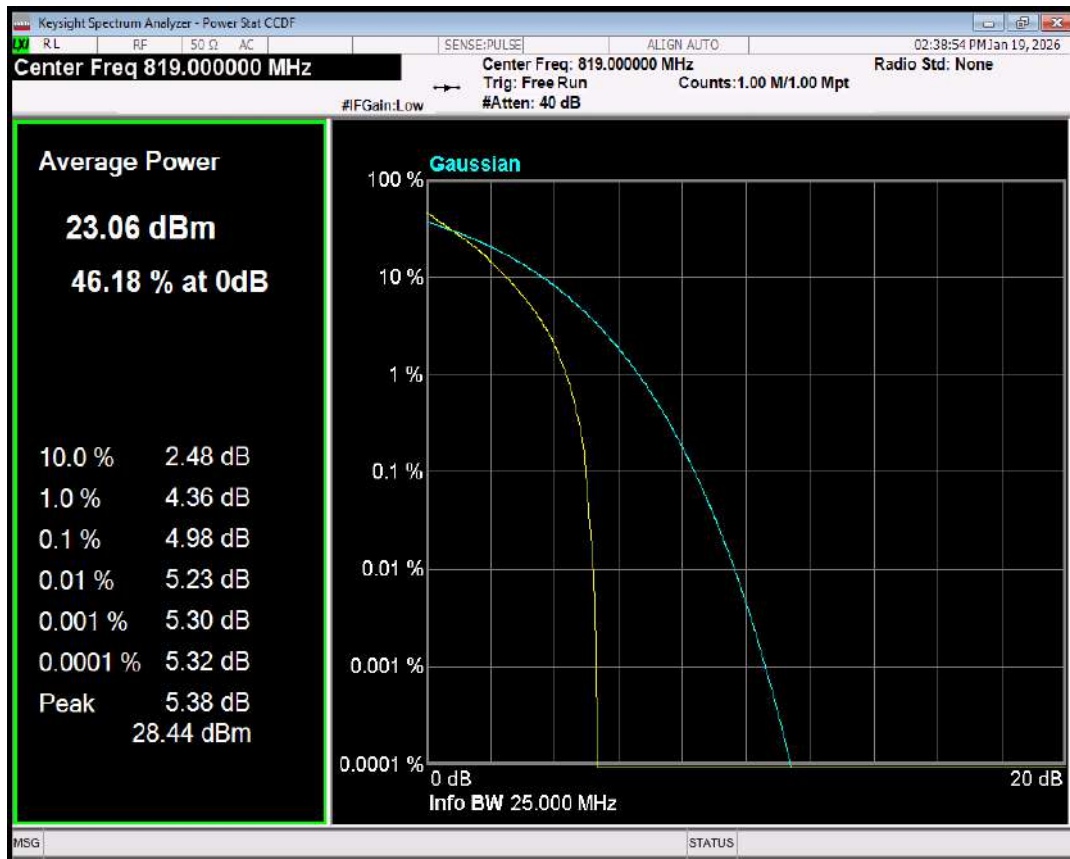
Band26(814-824) 16QAM BW=5MHz Channel=26740 RB Size=1 Position=#0
