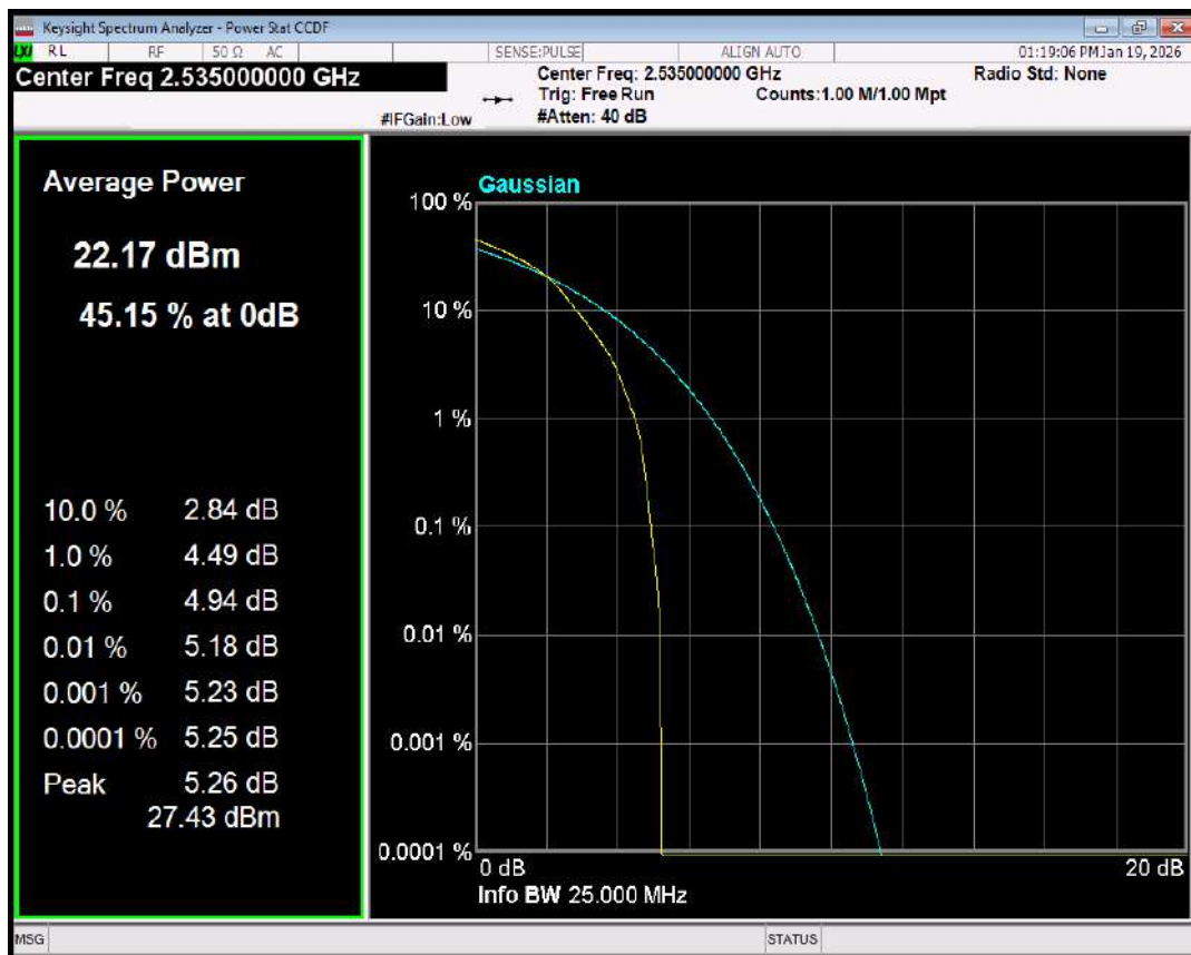
Band7 QPSK BW=15MHz Channel=21100 RB Size=1 Position=#0
