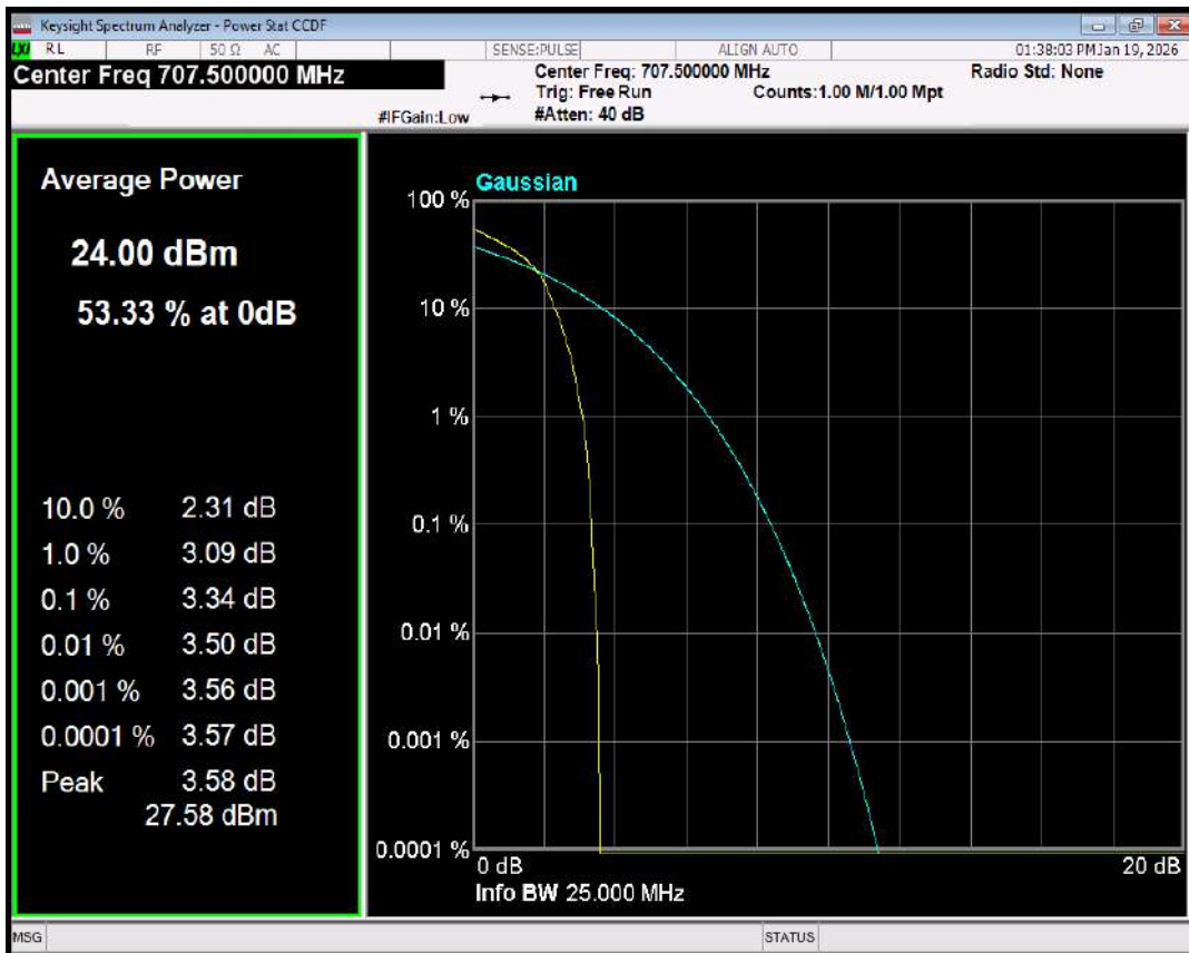
Band12 QPSK BW=5MHz Channel=23095 RB Size=1 Position=#0
