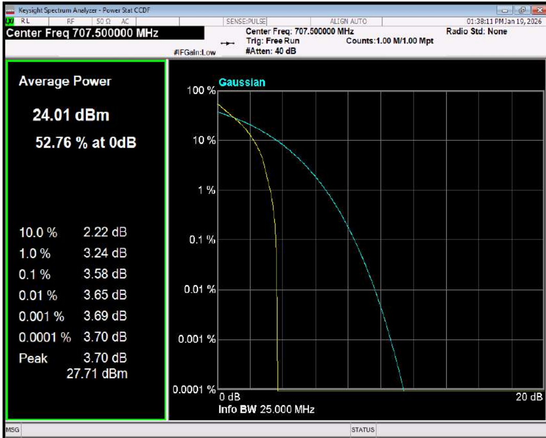
Band12 16QAM BW=10MHz Channel=23095 RB Size=1 Position=#0
