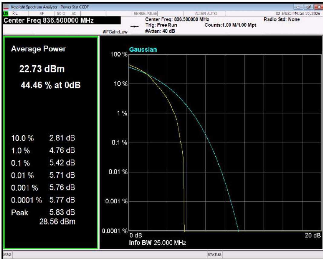
Band4 QPSK BW=1.4MHz Channel=20175 RB Size=1 Position=#0
