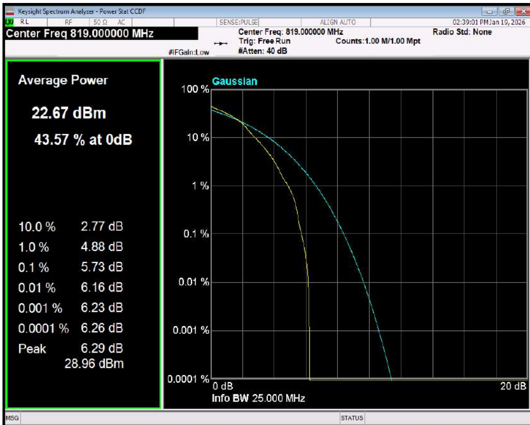
Band26(824-849) QPSK BW=1.4MHz Channel=26915 RB Size=1 Position=#0
