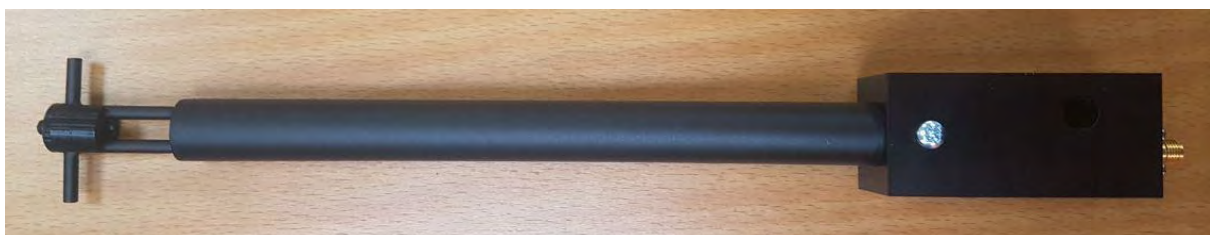
Figure 1 – MVG COMOSAR Validation Dipole
