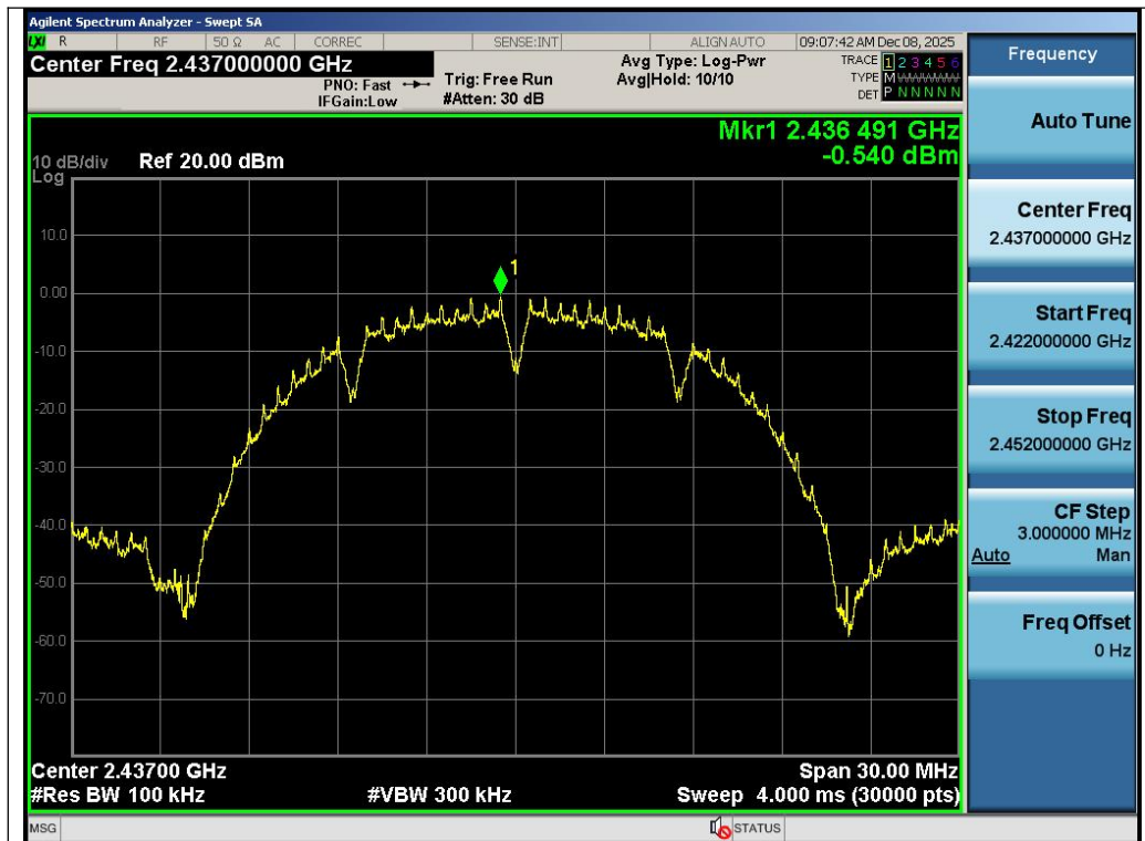
Test_Graph_802.11b_ANT1_2437_1Mbps_Lower Band Emissions
