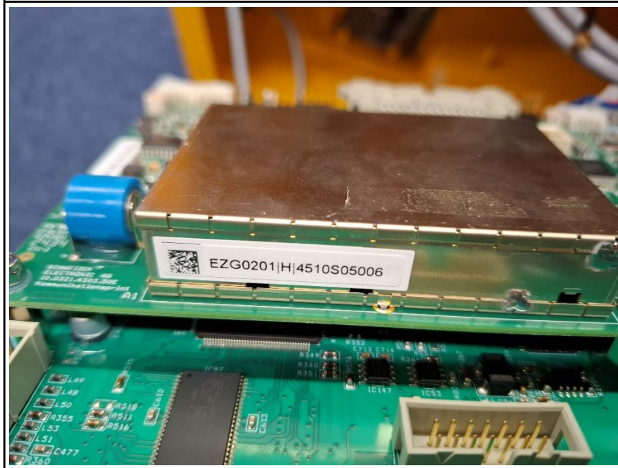
Radio unit with label and shielding
