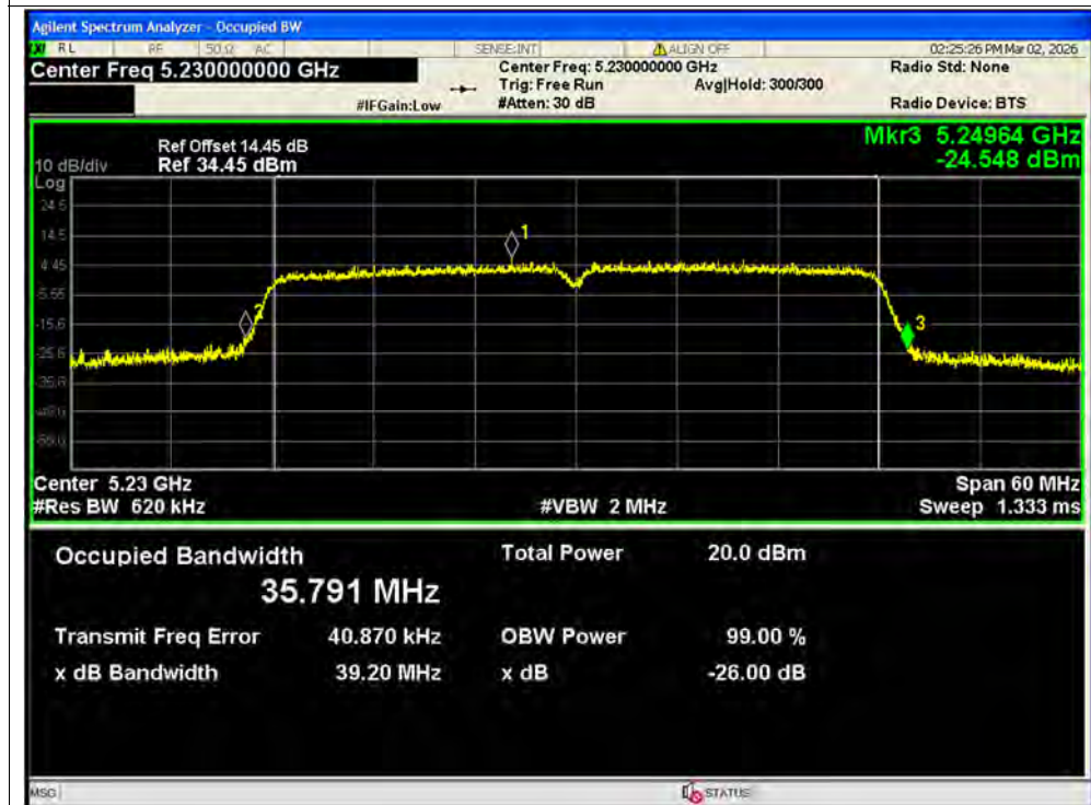
-26dB Bandwidth NVNT ac40 5230MHz Ant1 SISO
