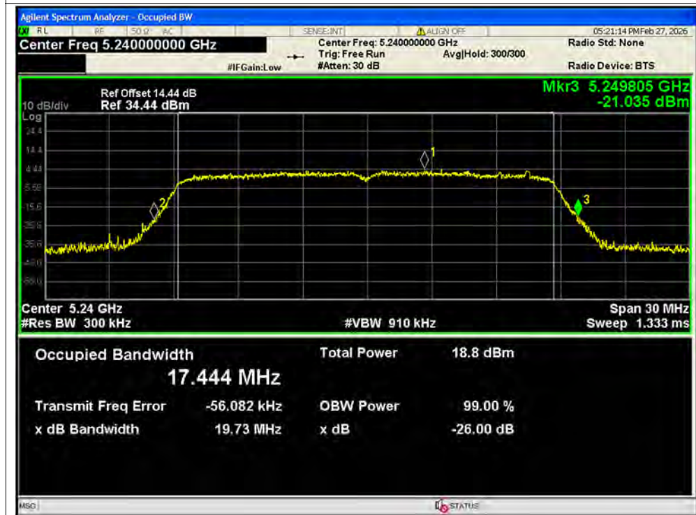
-26dB Bandwidth NVNT ac20 5240MHz Ant2 SISO
