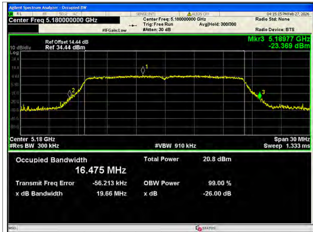
-26dB Bandwidth NVNT a 5180MHz Ant1 SISO
