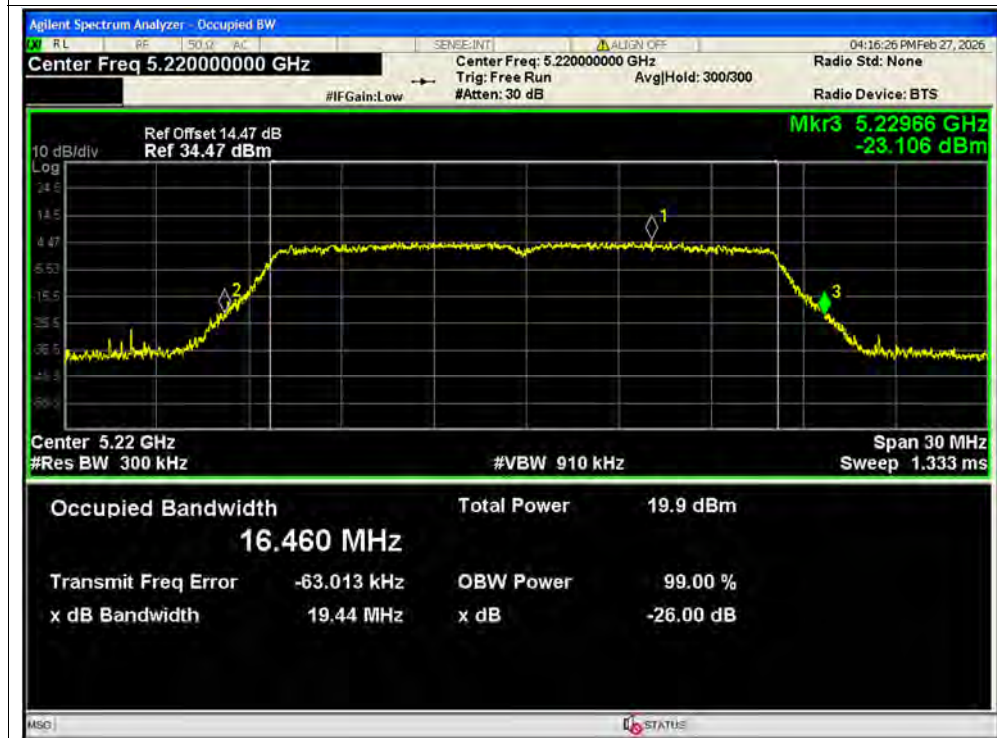
-26dB Bandwidth NVNT a 5220MHz Ant1 SISO
