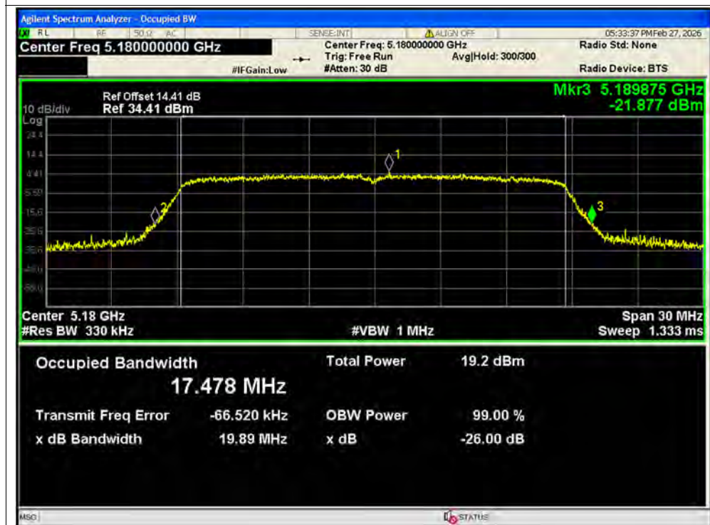
-26dB Bandwidth NVNT n20 5180MHz Ant2 MIMO
