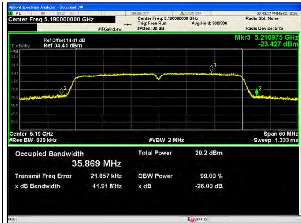
-26dB Bandwidth NVNT ac40 5190MHz Ant2 SISO
