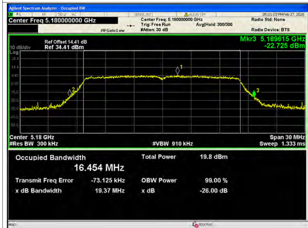
-26dB Bandwidth NVNT a 5180MHz Ant2 SISO
