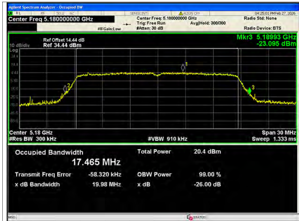
-26dB Bandwidth NVNT n20 5180MHz Ant1 SISO
