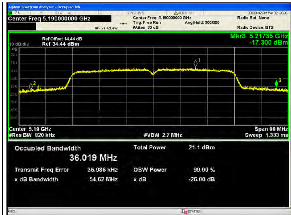
-26dB Bandwidth NVNT ac40 5190MHz Ant1 MIMO
