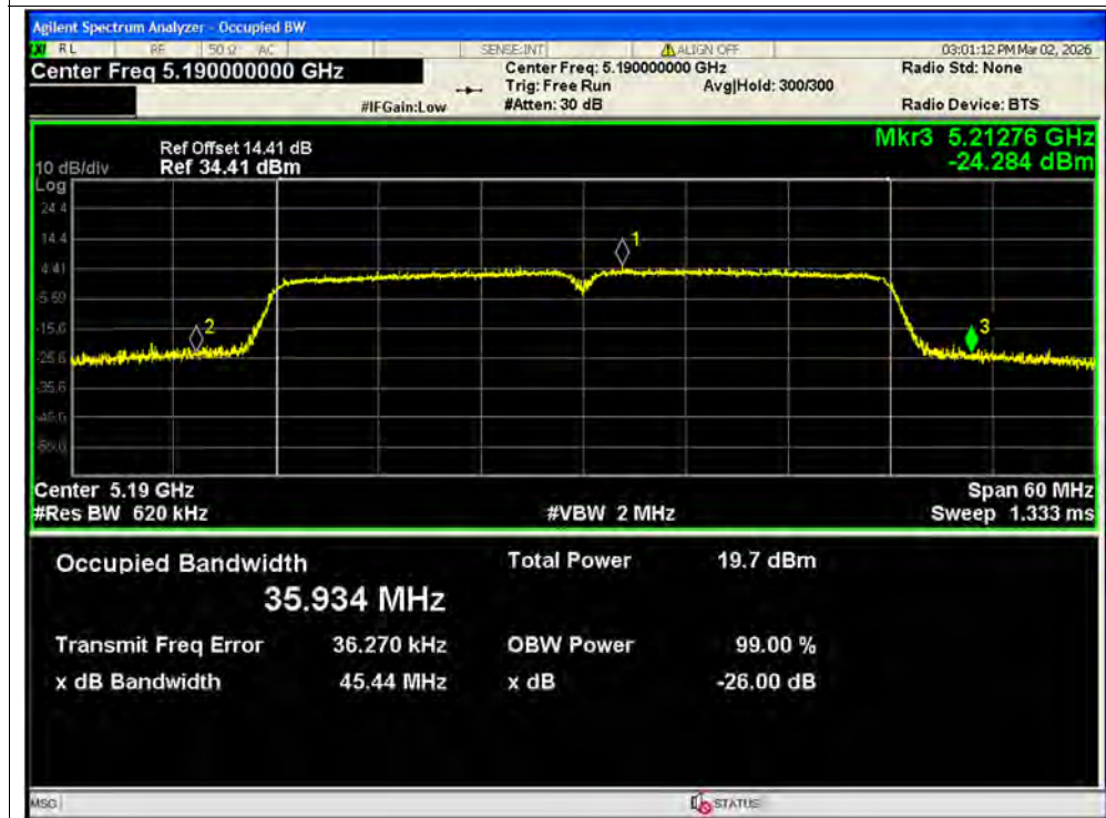
-26dB Bandwidth NVNT ac40 5190MHz Ant2 MIMO
