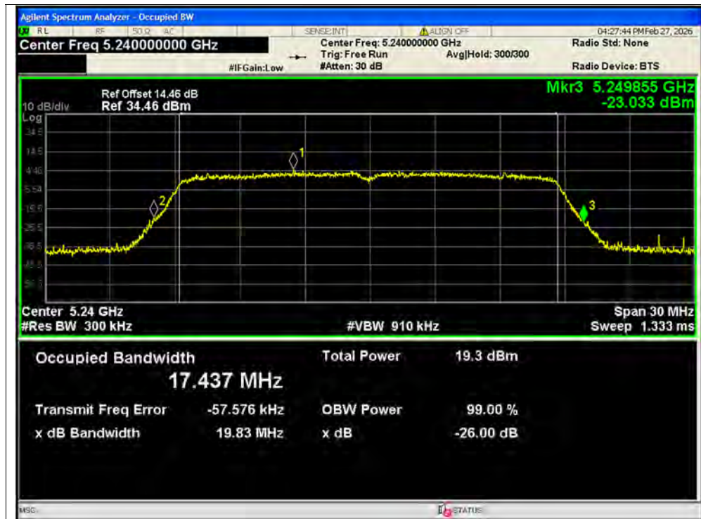
-26dB Bandwidth NVNT n20 5240MHz Ant1 SISO
