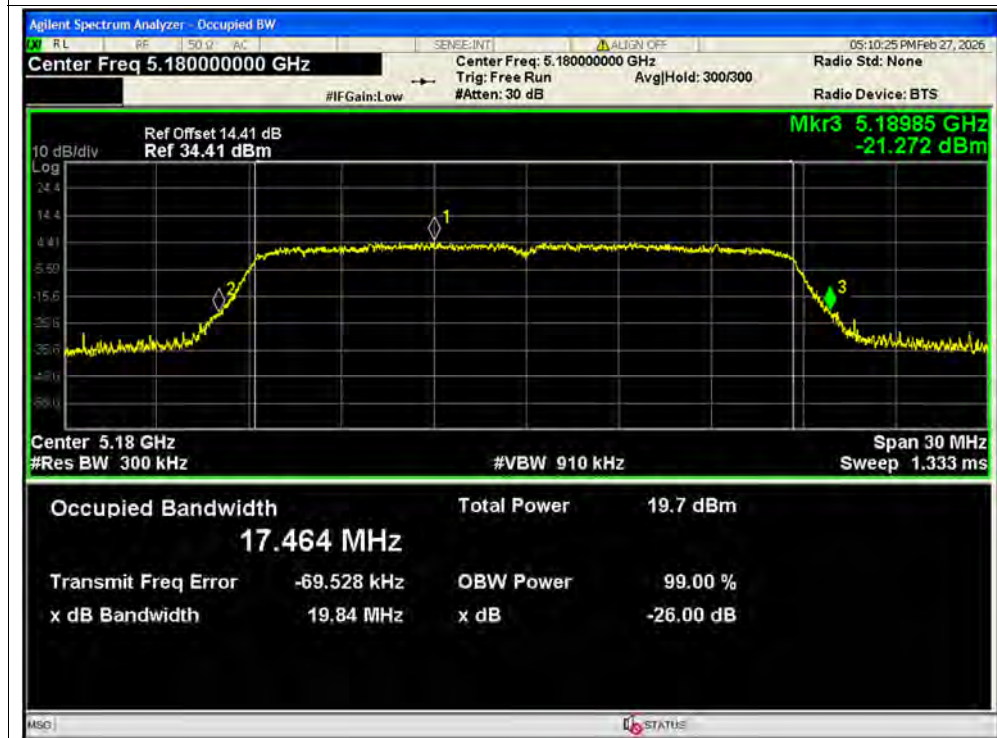
-26dB Bandwidth NVNT n20 5180MHz Ant2 SISO
