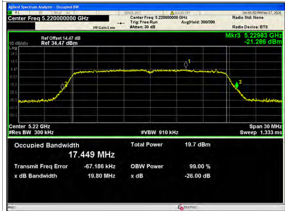
-26dB Bandwidth NVNT ac20 5220MHz Ant1 SISO
