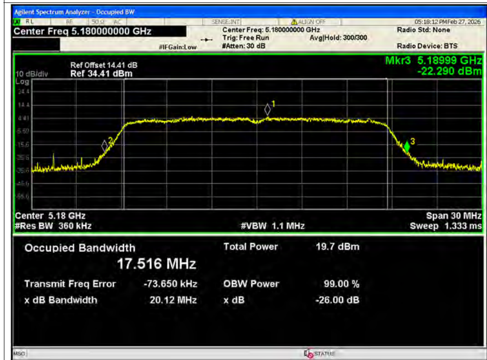
-26dB Bandwidth NVNT ac20 5180MHz Ant2 SISO
