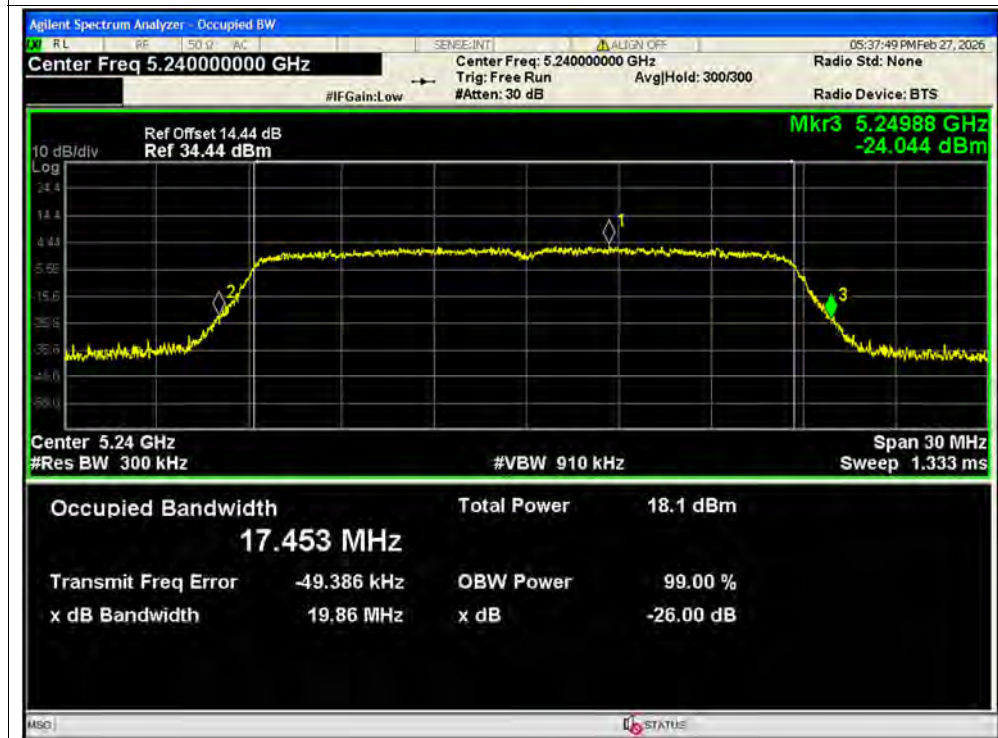
-26dB Bandwidth NVNT n20 5240MHz Ant2 MIMO
