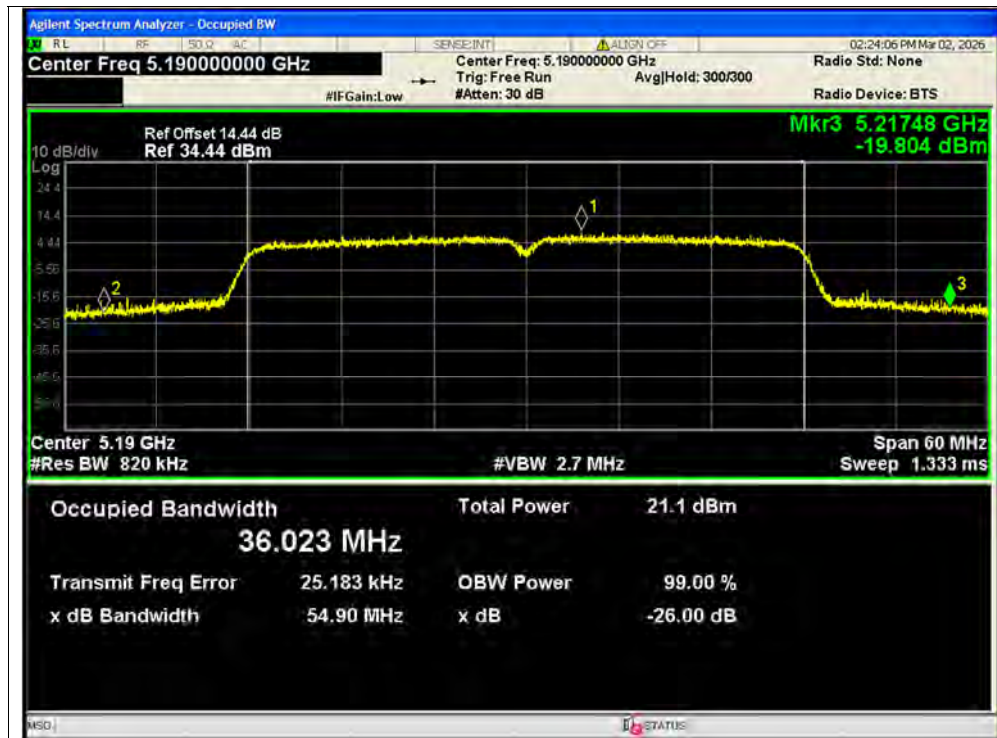
-26dB Bandwidth NVNT ac40 5190MHz Ant1 SISO
