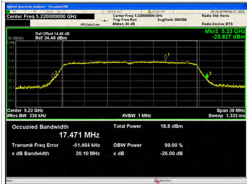
-26dB Bandwidth NVNT n20 5220MHz Ant2 MIMO
