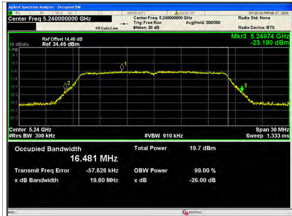
-26dB Bandwidth NVNT a 5240MHz Ant1 SISO
