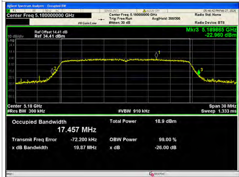
-26dB Bandwidth NVNT ac20 5180MHz Ant2 MIMO
