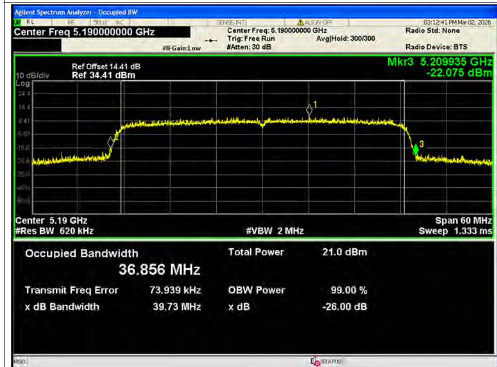
-26dB Bandwidth NVNT ax40 5190MHz Ant2 MIMO
