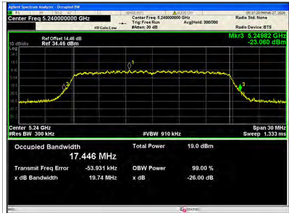
-26dB Bandwidth NVNT n20 5240MHz Ant1 MIMO
