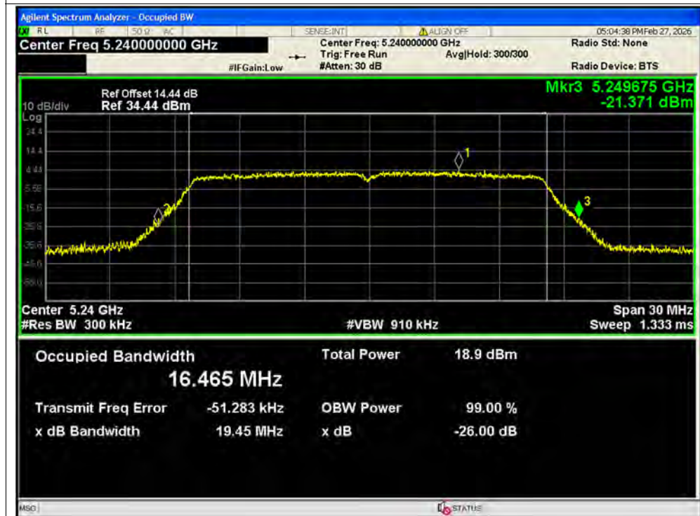
-26dB Bandwidth NVNT a 5240MHz Ant2 SISO
