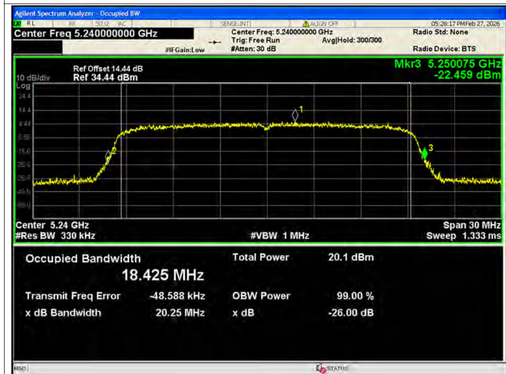
-26dB Bandwidth NVNT ax20 5240MHz Ant2 SISO
