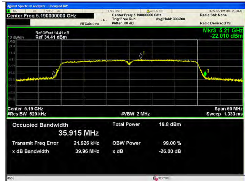
-26dB Bandwidth NVNT n40 5190MHz Ant2 MIMO
