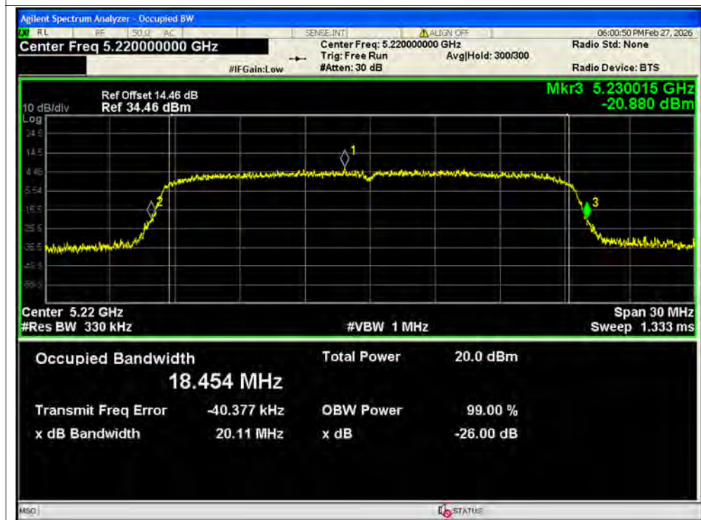
-26dB Bandwidth NVNT ax20 5220MHz Ant2 MIMO
