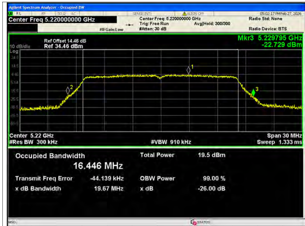
-26dB Bandwidth NVNT a 5220MHz Ant2 SISO
