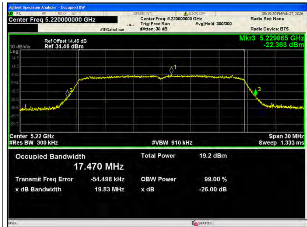
-26dB Bandwidth NVNT ac20 5220MHz Ant2 SISO
