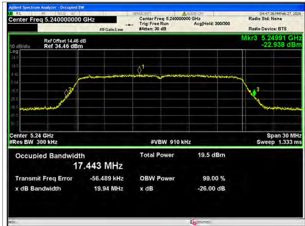
-26dB Bandwidth NVNT ac20 5240MHz Ant1 SISO
