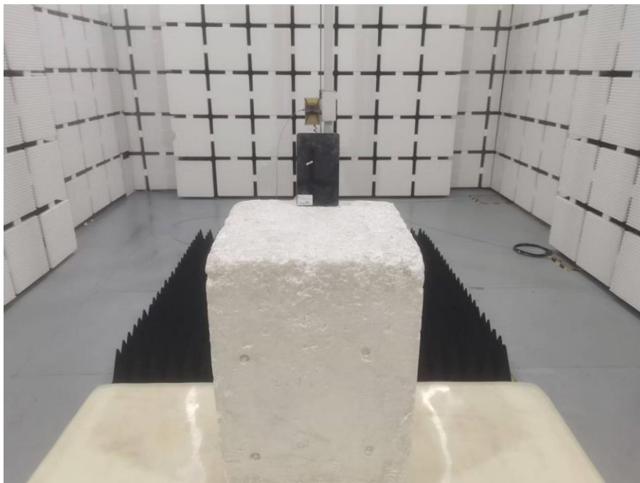
Set-up for Radiated Spurious Emission, Above 1GHz
