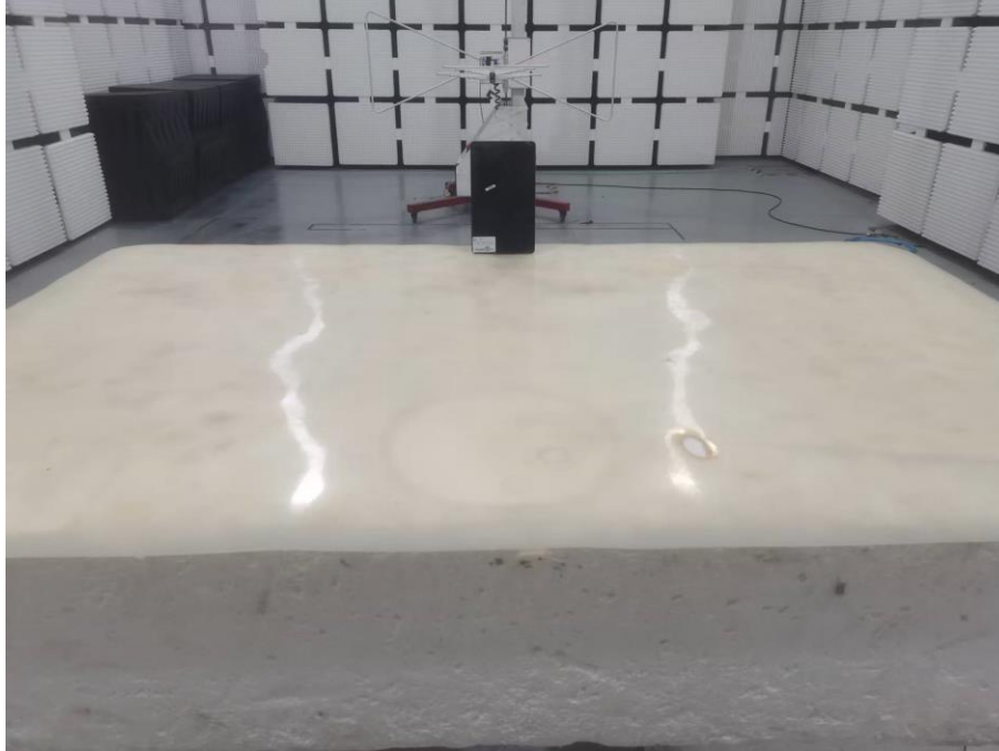
Set-up for Radiated Spurious Emission, Above 1GHz
