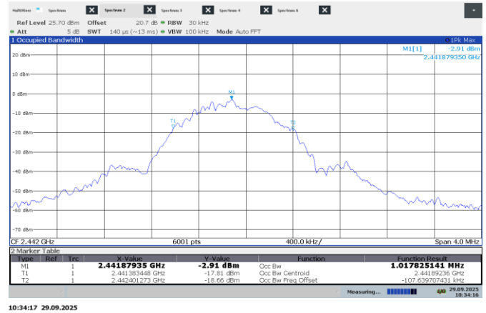
Figure 7.4-5: 99% occupied bandwidth on 802.11g, sample plot
