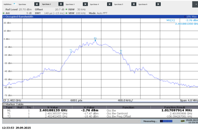
Figure 7.4-4: 99% occupied bandwidth on 802.11b, sample plot
