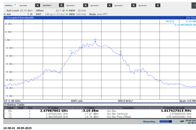
Figure 7.4-6: 99% occupied bandwidth on high ch.
