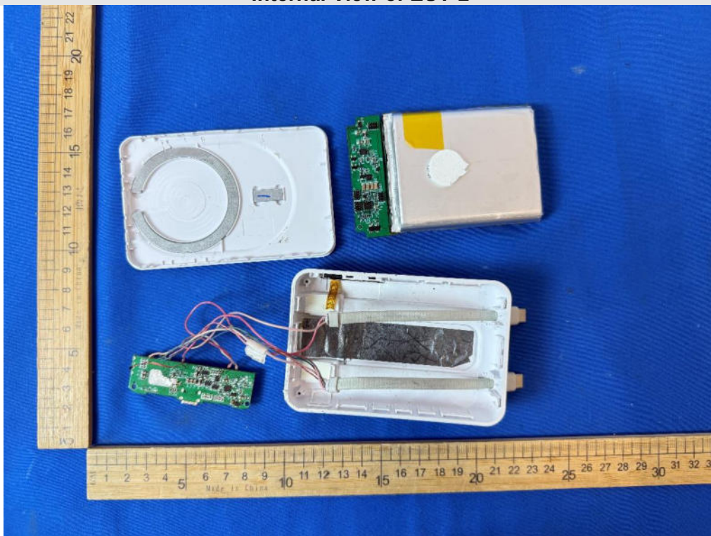
Internal View of EUT-2
