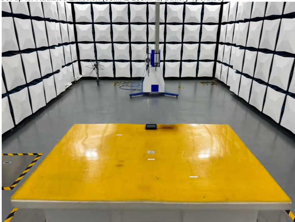
Set-up for Radiated Emission (200MHz-1000MHz, Battery operated)
