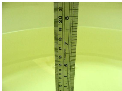
Fig 7.2 Photo of Liquid Height for Body SAR
