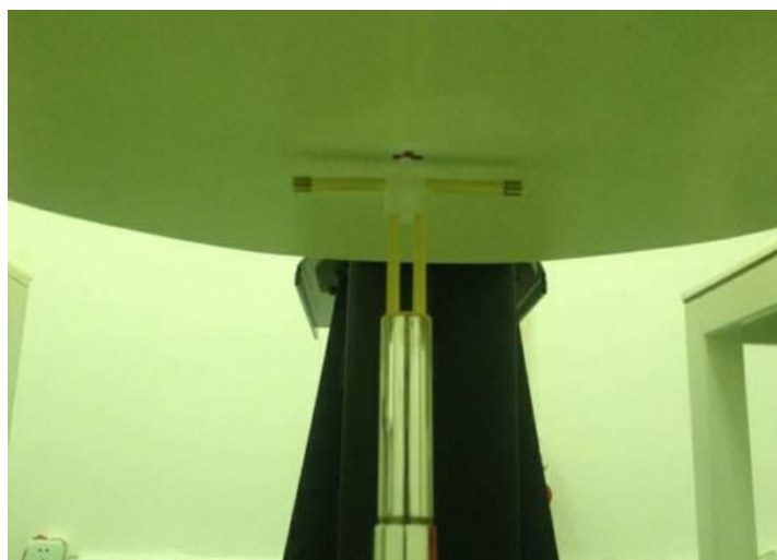
Photo of Dipole Setup
