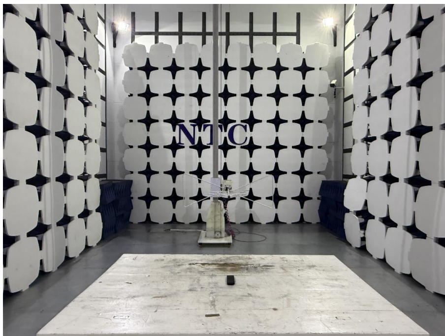
Photos of radiated emission test 30MHz – 1GHz
