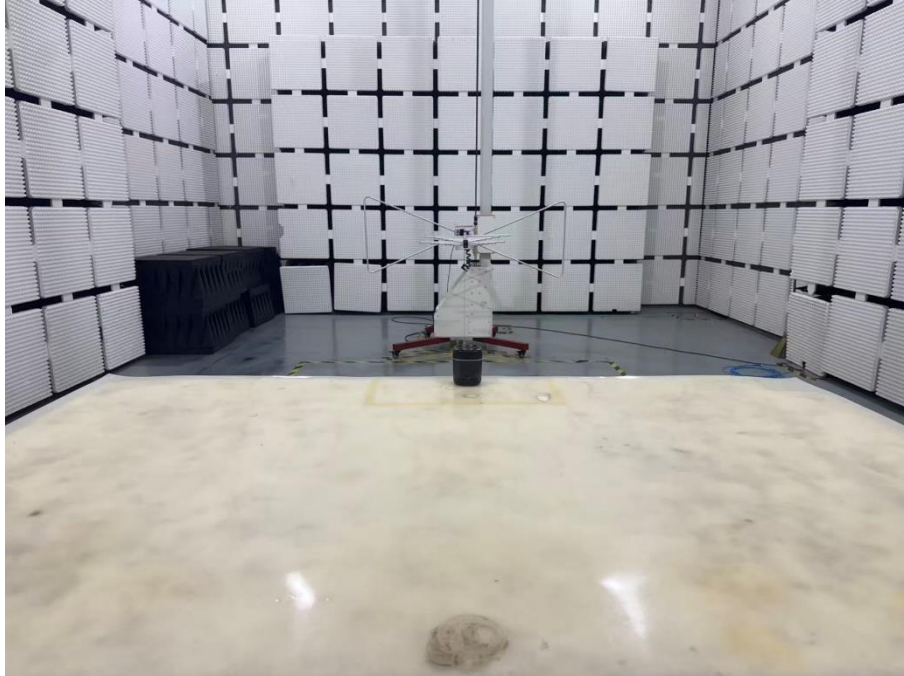
Set-up for Radiated Spurious Emission, Above 1GHz
