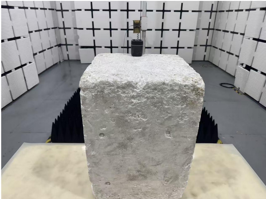
Set-up for Radiated Spurious Emission, Above 1GHz
