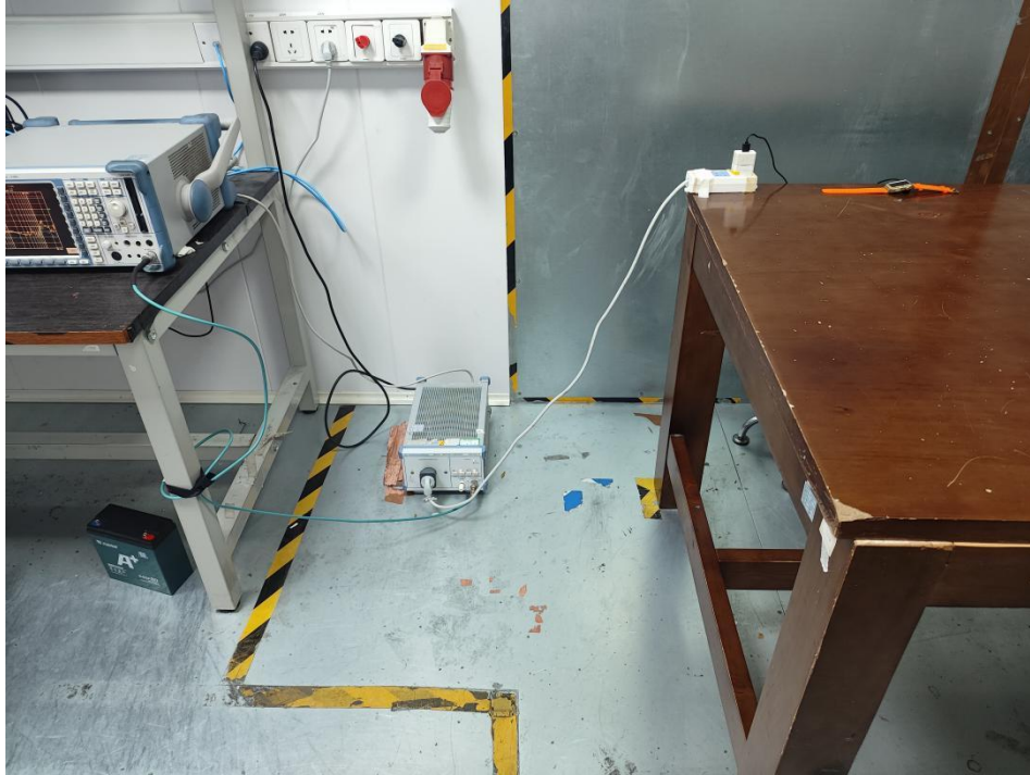
Conducted Emissions at Mains Terminals (150 kHz-30MHz)
