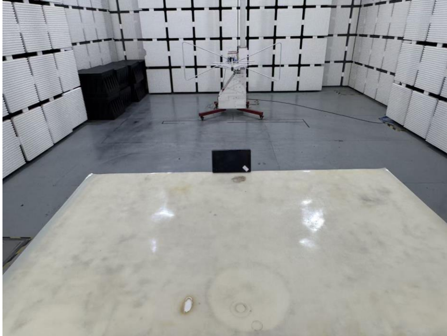
Set-up for Radiated Spurious Emission, Above 1GHz
