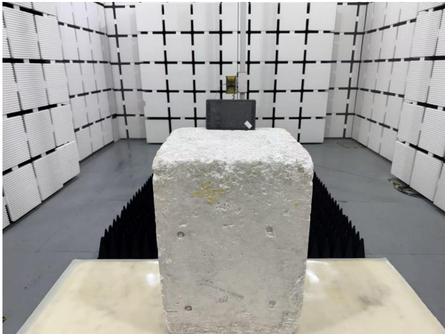
Set-up for Radiated Spurious Emission, Above 1GHz
