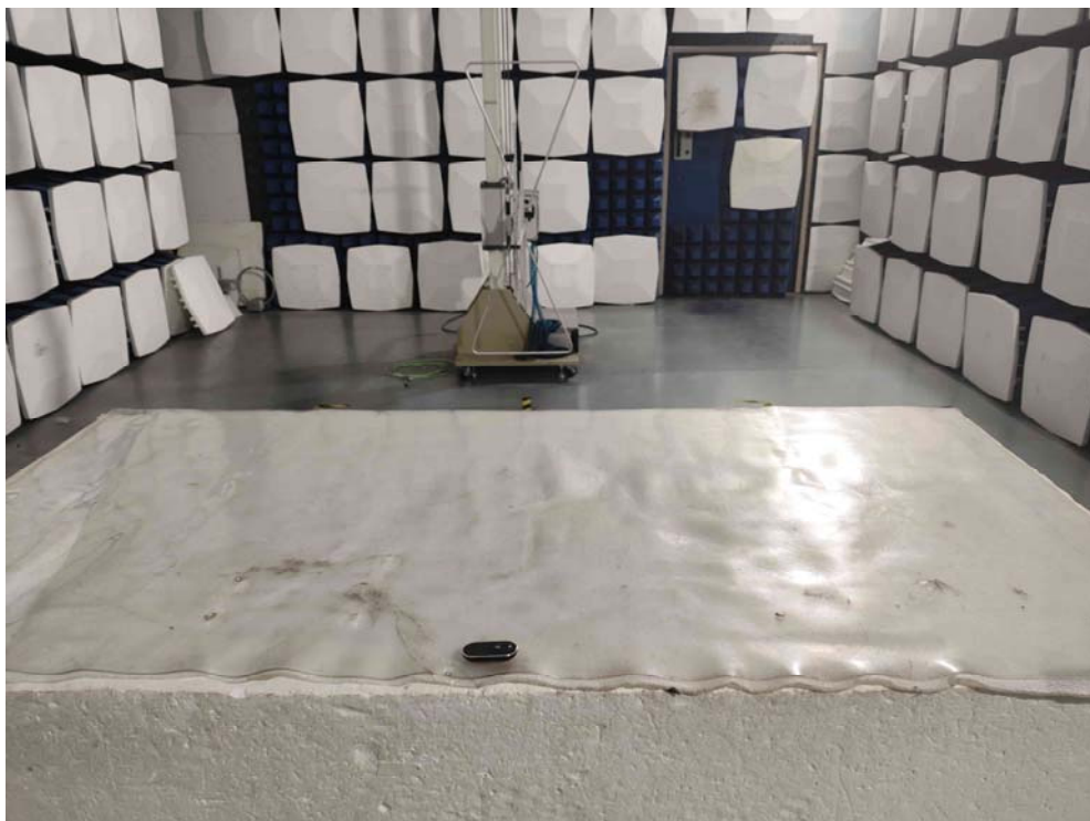
Radiated emission test view
